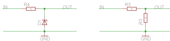
Figure 3.5: Level converter to clip the incoming voltage (left) or to scale the incoming voltage (right).
