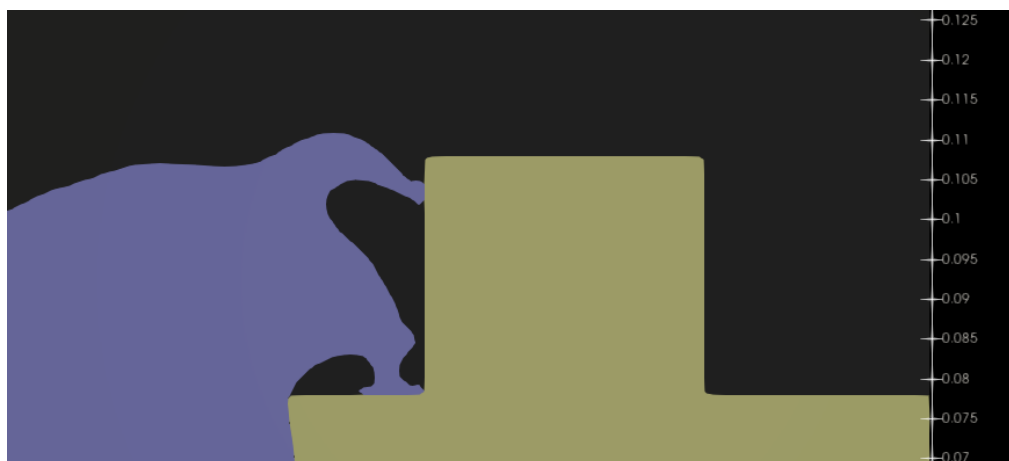
Figure 6.13: Freeboard exceedance height estimated for the 20m-simulation.
