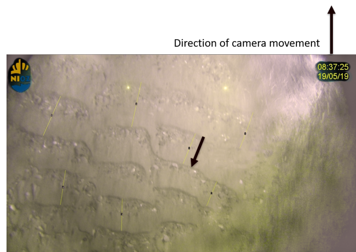
Figure 10. Still frame from video data. The black arrow in the frame indicates the direction of the sand ripples. The arrow above the frame indicates the direction of camera movement. Yellow lines were drawn in ImageJ to determine ripple orientation and length.
