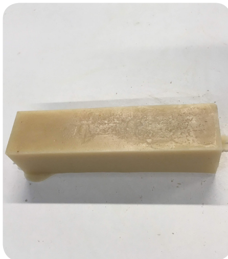
Step 5: Wax beam of 150*40*40 mm
