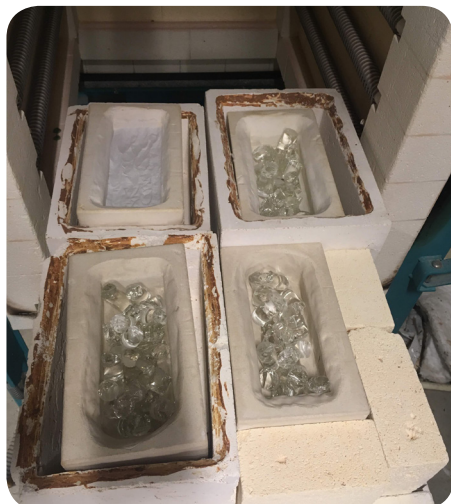
Step 19: Four moulds with borosilicate glass before entering the kiln
