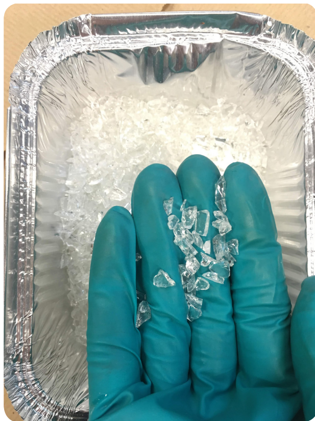
Figure 66 Borosilicate cullet of >2.3 mm < 5 mm
