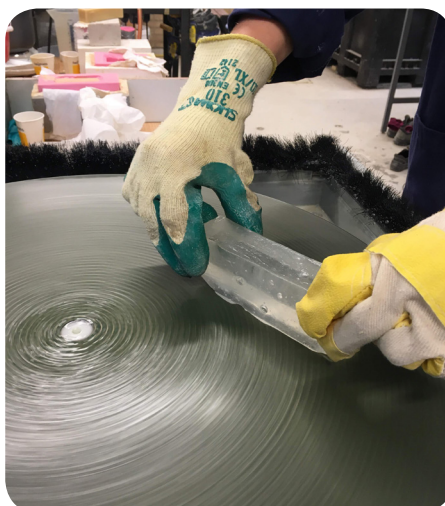
Step 17: Grinding the beam to the desired shape and for a smooth/transparent finish
