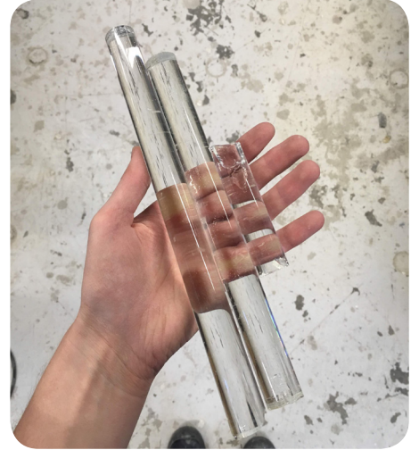
Step 12: Borosilicate glass rods by Schott
