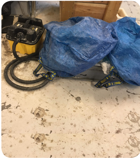
Step 10: Steaming the wax out of the Crystal Cast mould
