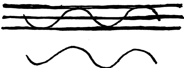
Figure 135 Instead of 1 curved beam, three straight beams are proposed
