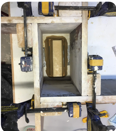
Step 7: Wax beam inside wooden planks for the creation of the Crystal Cast mould
