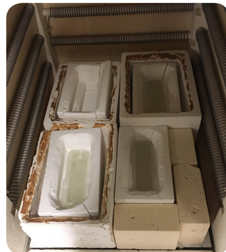
Step 21: Four moulds with borosilicate glass after firing in the kiln
