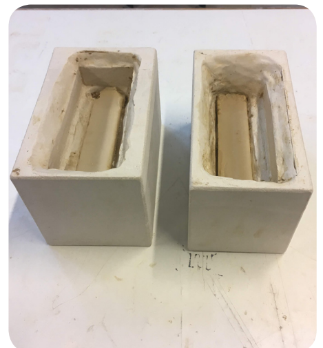
Step 9: Two Crystal Cast moulds with wax beam still inside
