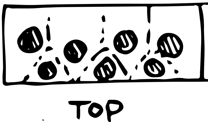
Figure 54 Specimen 3, placement of the rods in the mould, corresponding to air bubble patterns, top view
