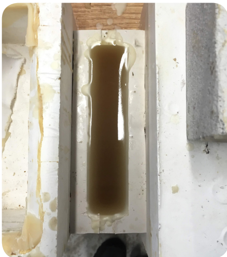
Step 4: Silicon mould with hot wax
