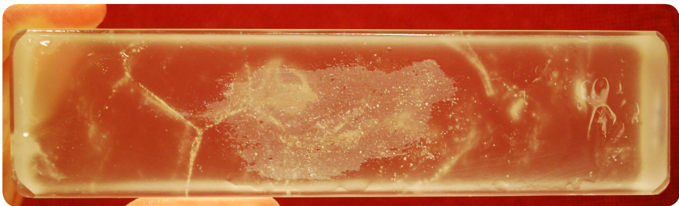
Figure 59 Specimen 5 air bubble entrapment
