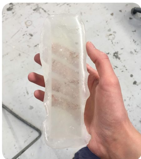
Step 16: A borosilicate glass beam of 150*40*40 mm, but with too much glass on the top part
