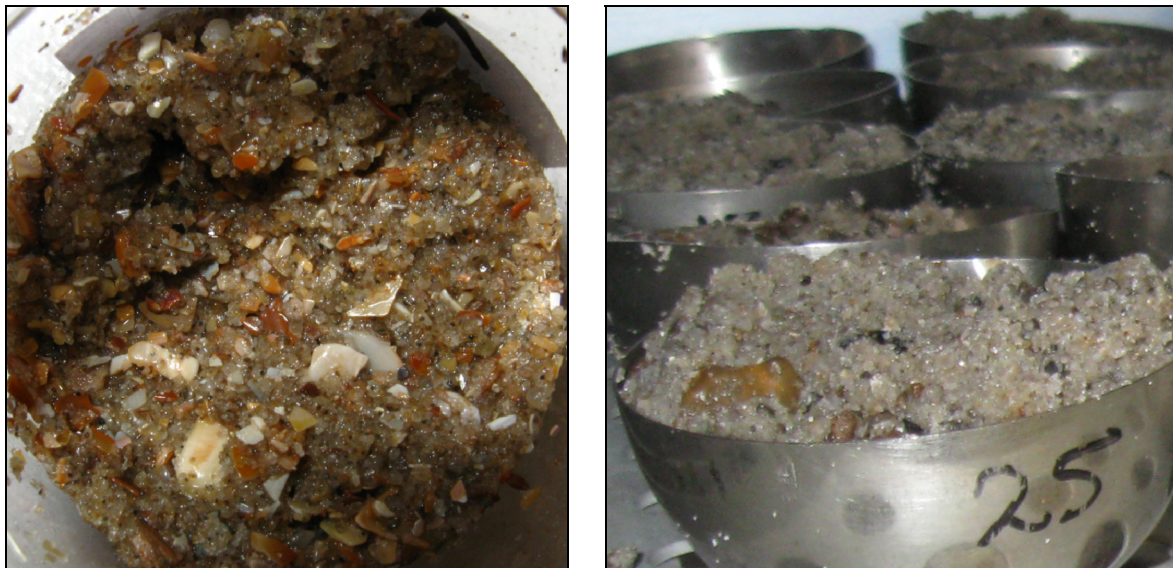
Figure 4-2 Sediment with shells from Egmond aan Zee (l) and with gravel from Hvide Sande (r)
