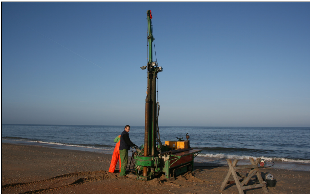
Figure 5-15 Drilling rig used to take deep samples from the subsurface
