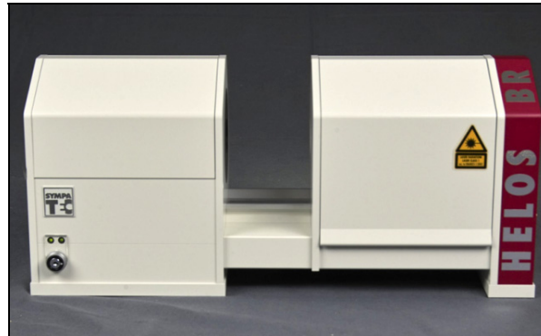
Figure B-4 The Laser Diffraction Sensor HELOS/BR, used during the analysis of the samples
