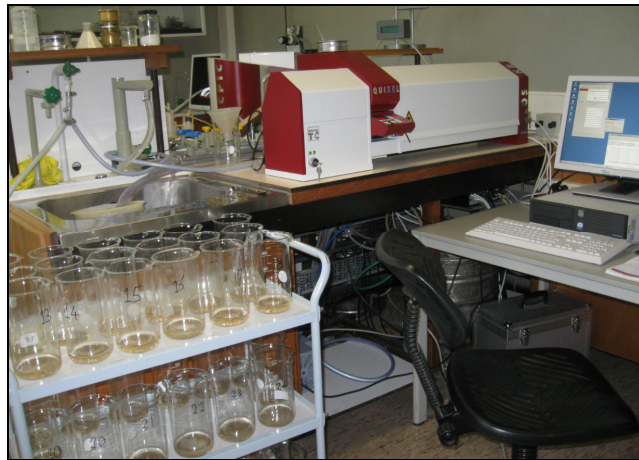
Figure 3-7 Test facility to analyse the sediment samples (laser diffraction sensor)
