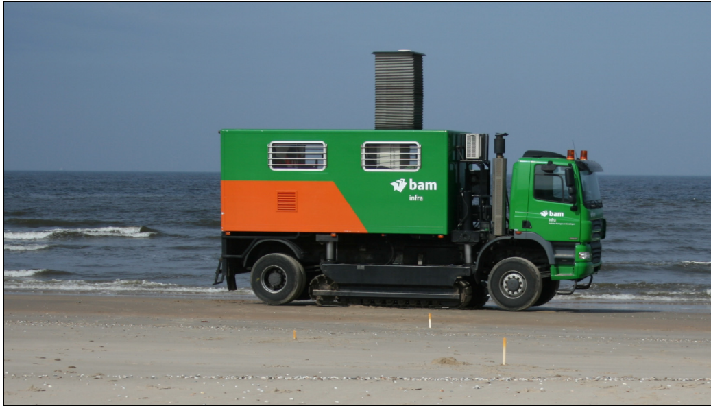
Figure 5-6 Cone penetration tests at the beach near Egmond aan Zee
