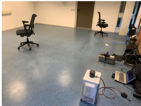
(c) Visualisation of the experimental setup in position four, showing the LiDAR sensor on its support as well as the smoke machine.
