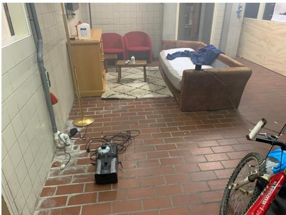
(c) The experimental setup with the LiDAR on the sofa and smoke machine positioned on the ground.
