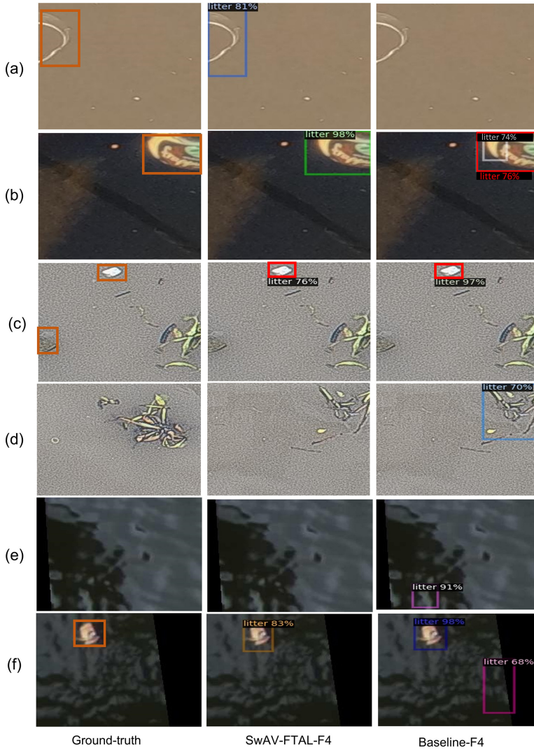
Figure 5.8: Detection results of the Faster R-CNN with ResNet50 backbone on Amsterdam, Groningen, and WUR-HCMC subsets using SwAV-FTAL-F4 and Baseline-F4 methods. The models were fine-tuned on the Train 100% subset. Both methods can detect litter items in (b), (c) and (f), and only the SwAV-FTAL-F4 method can detect the litter item in (a). Common misdetection of the Baseline-F4 method includes identifying organic materials (d) and wave ((e) and (f)) as litter. Ground-truth litter is shown in red bounding boxes in the top row.
