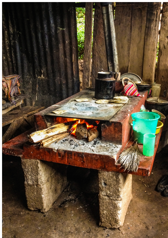
Figure 3.2: Flat iron top cookstove Photo by Diego Quan in the community El Zapotalito , 2016
