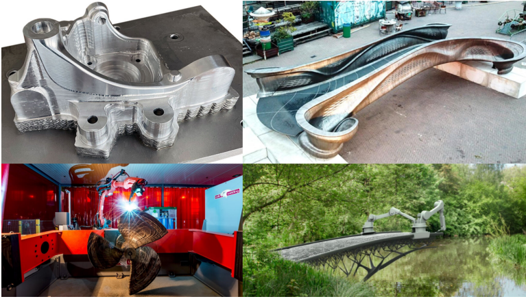
Figure 1.2.: Components manufactured using WAAM. Top left: A WAAM produced engineering component (Courtesy MIGAL). Top right: World's first metal additively manufactured bridge [59, 82] (Courtesy MX3D). Bottom left: A marine propeller is under construction using WAAM (Courtesy RAMLAB). Bottom right: Artistic illustration of a self-support robotic manufacturing bridge (Courtesy MX3D).
