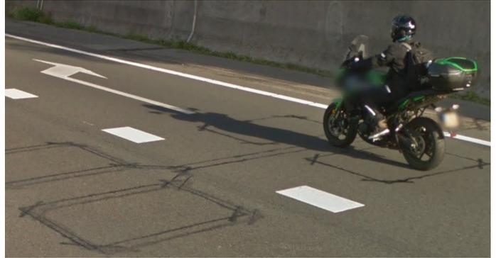
Fig. 4: A motorcycle passing a detection loop<sup>6</sup>.
