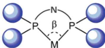
Figure 2.2: Schematic representation of the bite angle ( \beta ) in a pincer metal complex.
