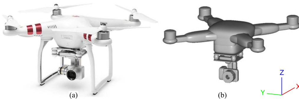
Figure 4.1. DJI Phantom III UAS used in impact modelling: (a) real-world system and (b) multibody system (MBS) model developed in MADYMO [11]. The two landing skids are neglected in the MBS model since they are such flexible that their impact effect is negligible [11].
