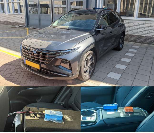
Fig. 4. The test vehicle, a Hyundai Tucson (top), equipped with a double antenna GPS (bottom left) and IMU system (bottom right) for measuring driving performance of human drivers
