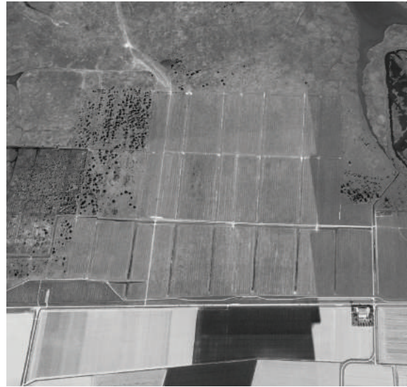
Fig. 51b: Gradual change from marshland to polder drainage pattern, Lauwersmeer (Google maps)
