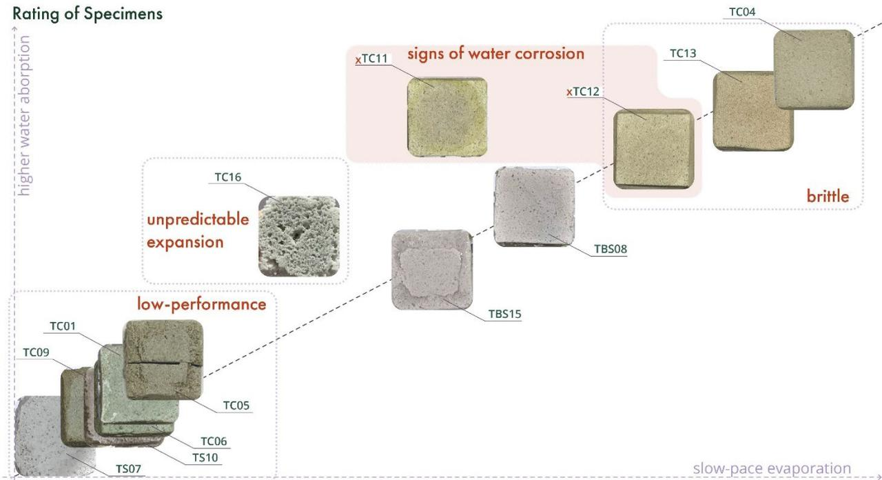
Figure 82. Diagram illustrating the findings of all the conducted tests, together with observations made along the process.
