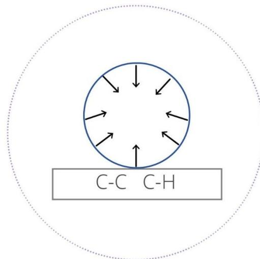
Appendix\_Figure 13. Diagram showing the water drop maintaining its spherical shape, without being absorbed by the hydrophobic solid. Image Source: Own.
