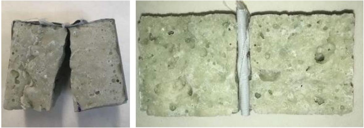
Figure 25. Photograph of the element after conducting the splitting experiment.  $F_{max}$  (N): 4478,62
