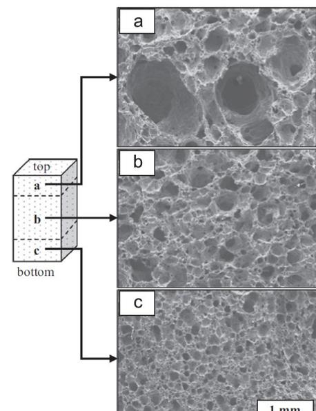
Figure 33. SEM micrograph of a specimen with panel CRT glass, with calcite foamed at 700°C for 15 min, presenting differences in the pore size and network along its height.
