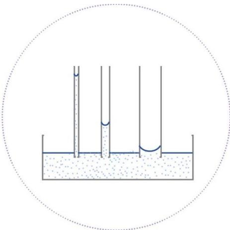
Appendix\_Figure 11. Diagram showing how smaller diameter pores are able to transfer the liquid further, by rising.
