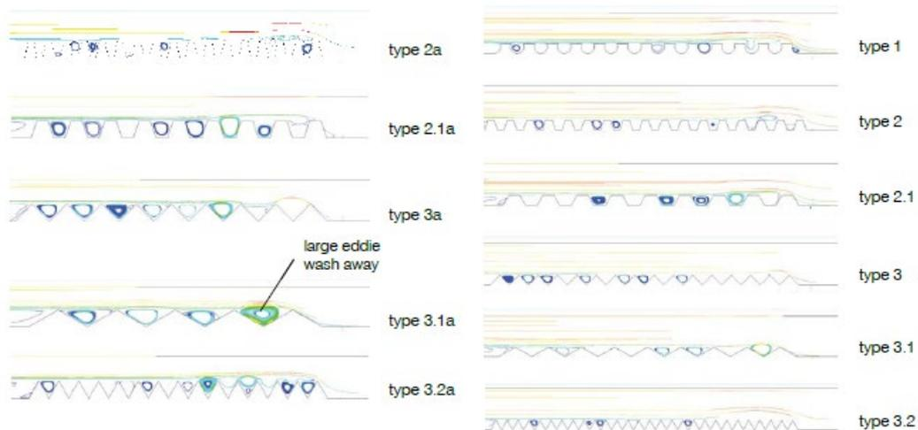
Figure 86. Streamline vertex diagram of CFD Simulations for micro-grooves geometry, inlet velocity set to 5m/s. Out of these tested formations, every time the best ones proceeded to the next detailed stage for simulations, by changing the section of the grooves.
