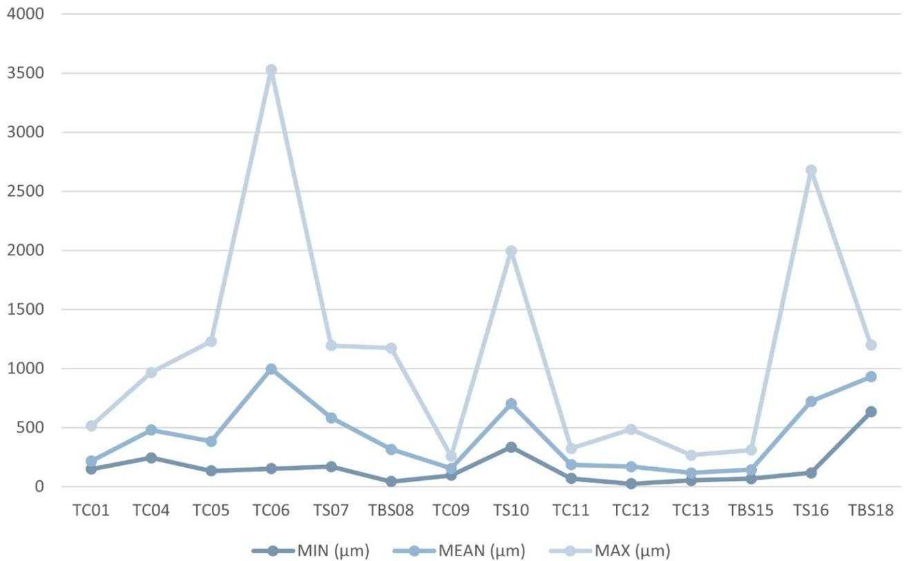
Chart 1. Lined-chart illustrating the pore sizes values of the polished surfaces of the cubic samples that were tested microscopically. Apart from the mean, the greatest range in sizes can be identified in the specimens TC06, TS10 and TS16, showing an uneven pore-distribution.
