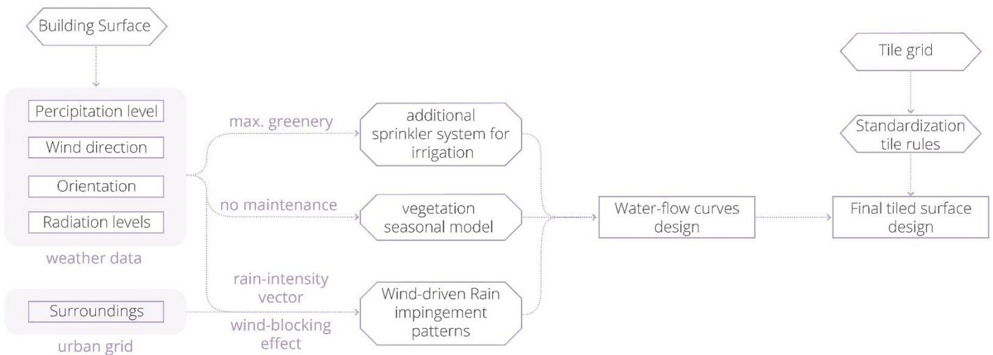
Figure 100. Decision flowchart regarding the general design of a surface in the urban environment, based on the bioreceptive design guidelines, regardless the final application product. This process can be applied both for roof, façade or acoustical tiles.
