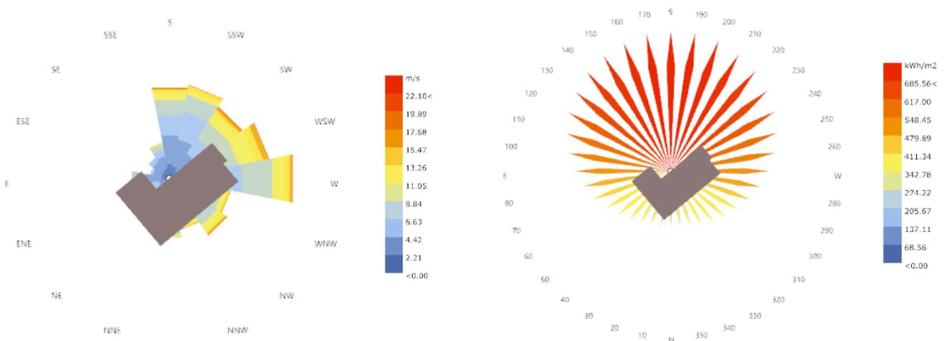
Figure 101. Wind rose (left) & radiation annual analysis (right) from the Montevideo tower in Rotterdam. South is oriented at the top. From these two diagrams, it is shown that the principle wind direction is the SW, while the radiation levels are important in combination with an analysis of the microorganisms' light needs.
