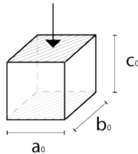
Figure 77. Diagram illustrating the specimens' measurements in relation to the applied force-surfaces.
