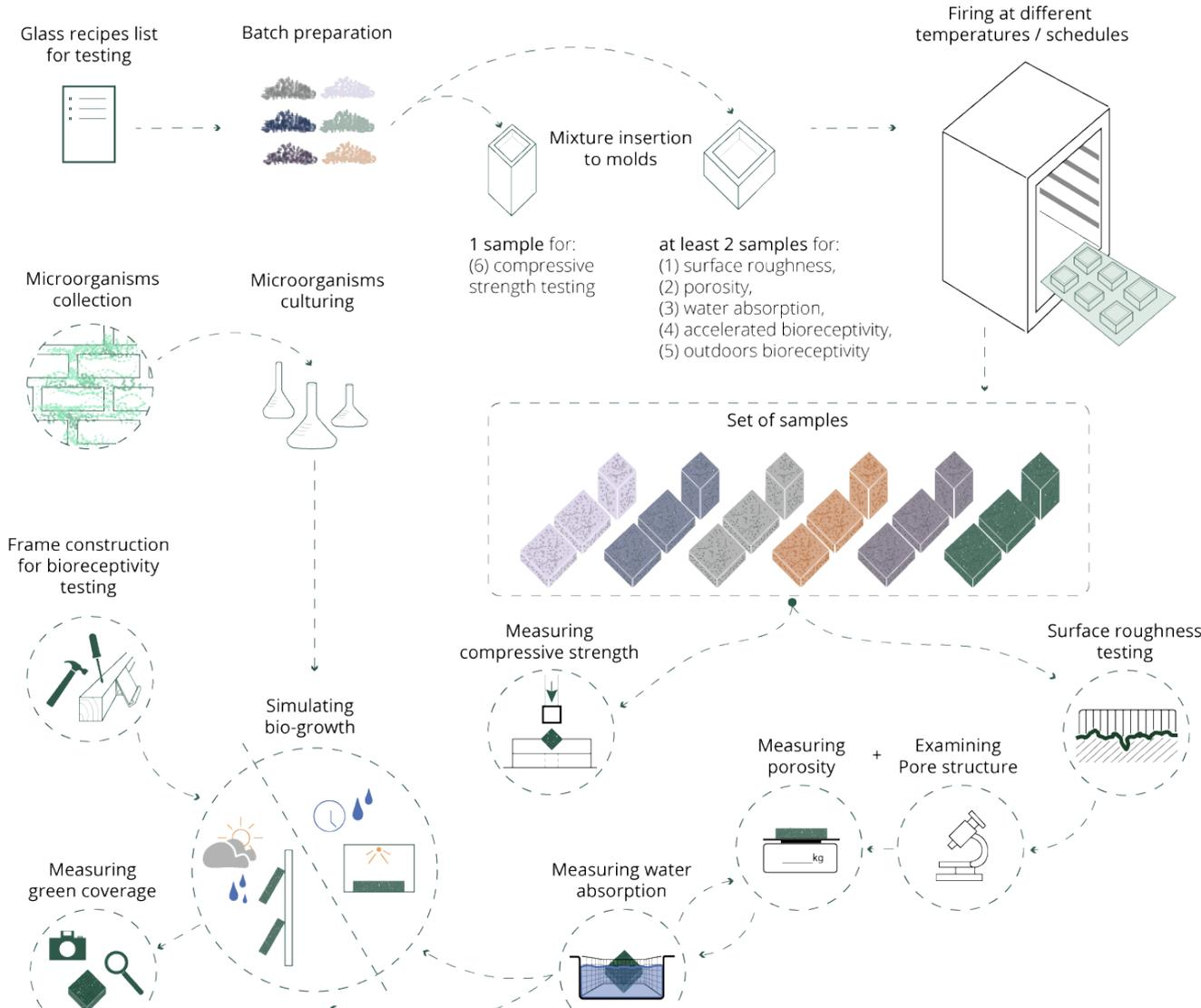
Figure 2. Infographic describing the 2<sup>nd</sup> part of the methodology - the experimental analysis - where the different samples are going to be tested for their properties and bioreceptivity potential.
