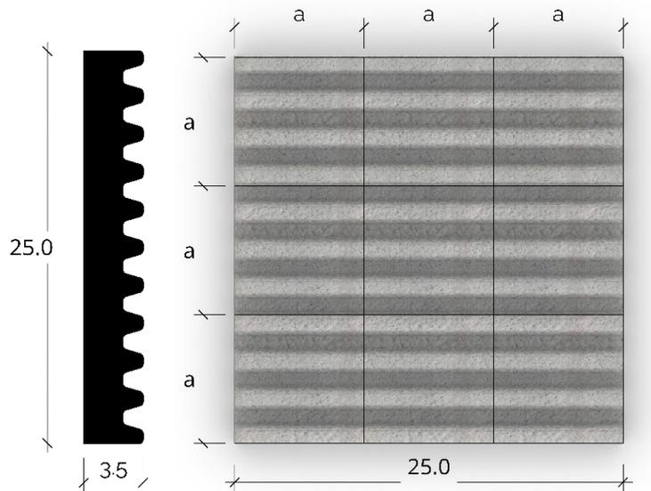
Figure 103. The case-study tile at its initial design phase with only the microgrooves engraved for microorganisms' anchorage and the division
