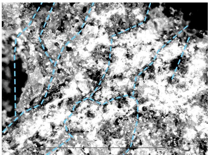
Figure 54. Connection route from the outer surface identified in a microscopic image of TC05, vertically sliced.
