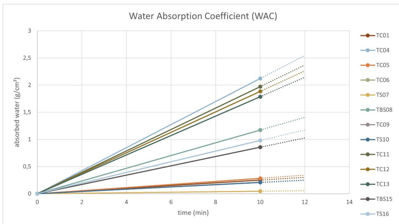
Chart 4. Isolated linear part of the absorption curve to measure WAC.
