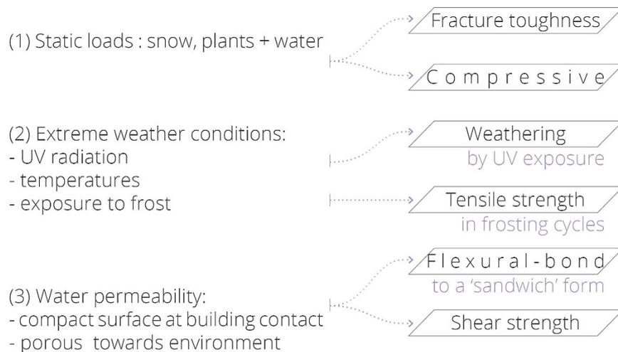
Figure 90. Identified critical points for the material based on the application's demands and the series of needed testing to provide the answers for the allowable product's specifications, adjusted for bioreceptivity. Image Source: Own.
