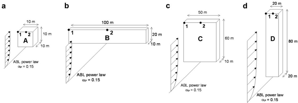
Appendix\_Figure 16. Different volumetric case studies to analyse the wind-blocking effect. (a) low-rise cubic building, (b) wide medium-rise building slab, (c) high-rise building slab, (d) tower building. Image Source: Blocken B. et al. (2013).
