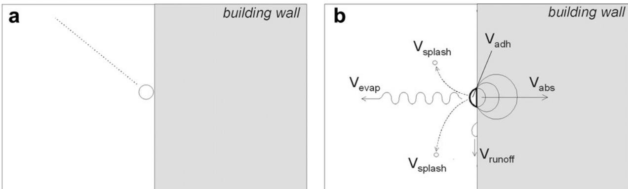
Appendix\_Figure 18. Diagram illustrating the separate phases of the wind-driven rain analysis. (a) defining the wind-driven rain intensity and pattern, (b) wall response at the raindrop. Image Source:
