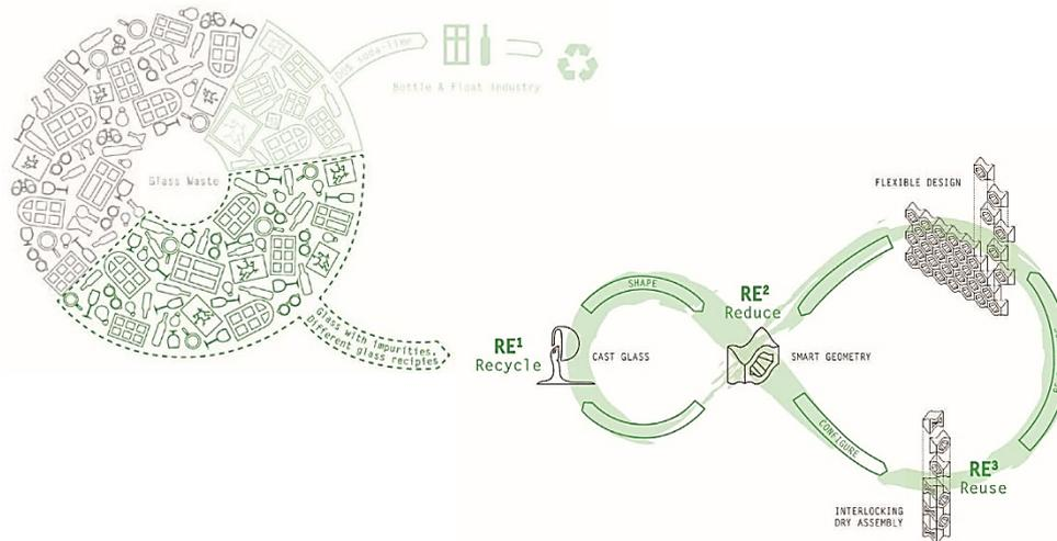
Figure 21. Diagram illustrating the portion of unutilized glass waste that can be exploited through the kiln-casting method in the building industry, by the proposal of Re<sup>3</sup> glass, suggesting a circular use with dry-assembling interlocking components.
