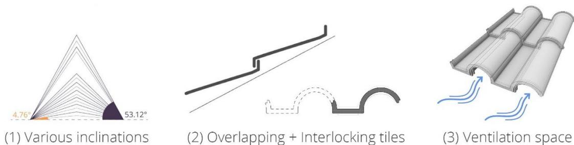
Figure 91. Diagram describing the primary set of design guidelines for roof tiles, forming the final input together with the boundary conditions for designing the product. Image Source: Own.
