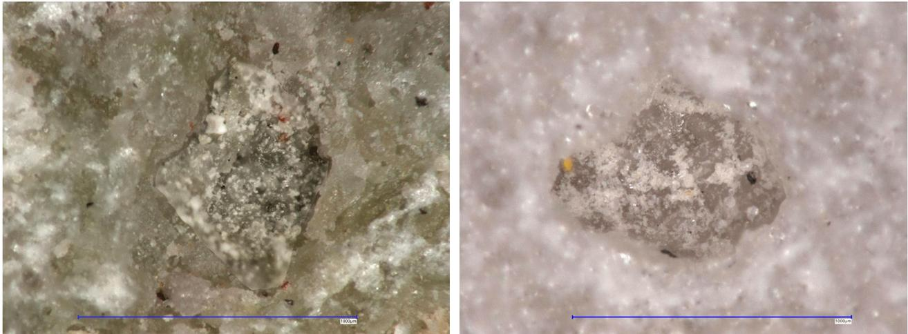
Figure 61. Microscopic image of TC05 (on the left), TS10 (on the right), calibrated to capture the depth of the pore. TC05: Irregular pore size of max dimensions: 613 x 823µm, TS10: 835 x 686µm.
