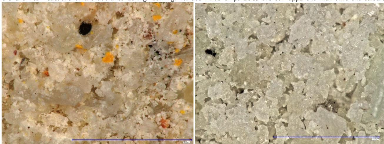
Figure 58. Microscopic images of TC04 & TC13, at different zoom scales (x200 & x150), depicting the range in sizes of the solid-pore matrix due to different percentages of foaming agent (10% & 3%). Yellow-coloured particles captured in TC04 are either contamination for waste in the Cyclon mix or from the saw-cutter in the cutting process in Stevin Lab II, in TU Delft.
