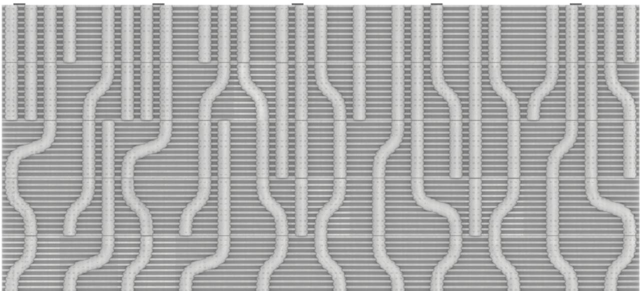
Figure 104. Façade fragment of 2,75 m length by 1,25 m height, as a design example of combining the standardized tiles.
