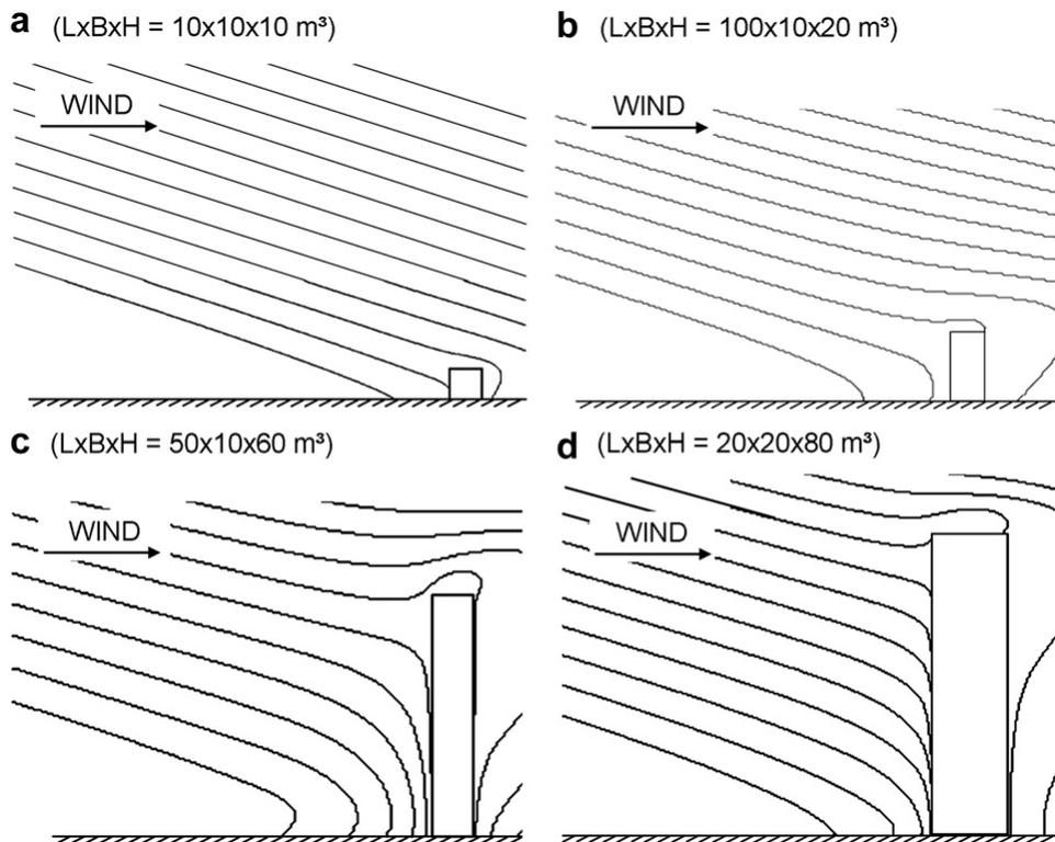
Appendix\_Figure 17. Wind flow pattern in the four different case studies, formed by rain trajectories of 1mm diameter raindrops, with a wind speed of 10m/s. Image Source: Blocken B. et al. (2013).
