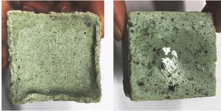
Figure 71. Sample TC06 showcasing similar effect with TC09, however, only the wider pore sizes seem to transfer the water into the sample.
