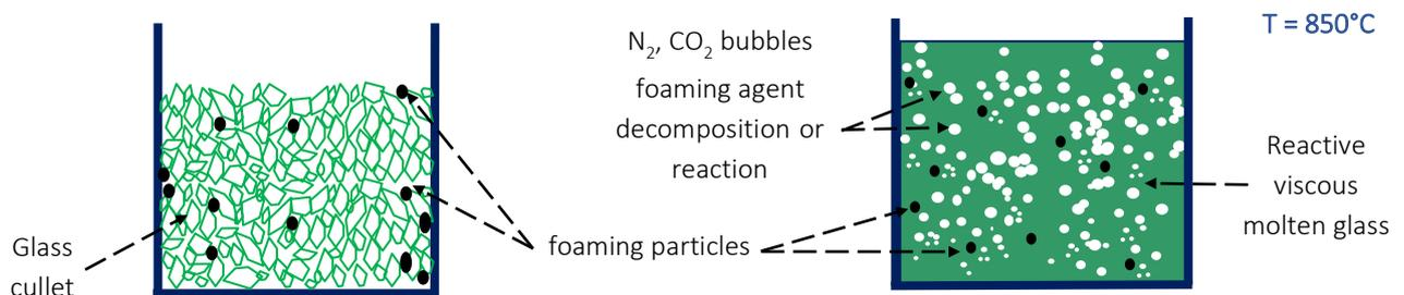
Figure 30. Diagram explaining the formation of foam glass out of glass powder mixed with foaming agent.
