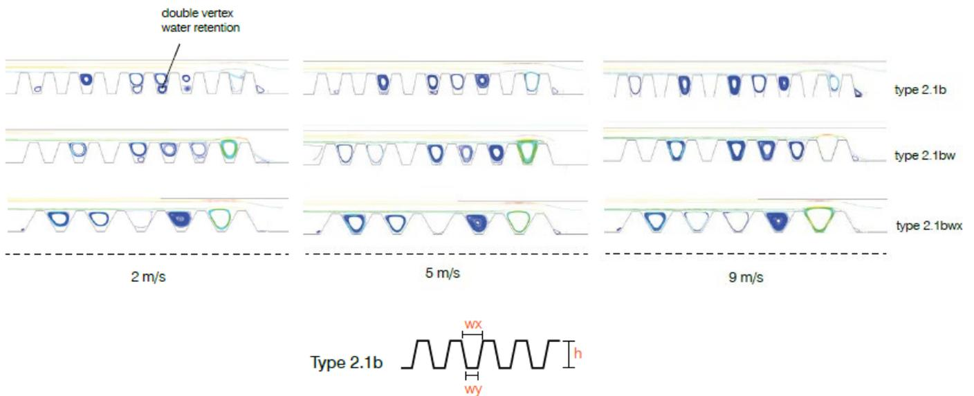
Figure 87. Streamline vertex diagram of CFD Simulations, with three different inlet velocities (from left to right): 2, 5, 9 m/s, illustrating the effect of altering the width of the groove geometry. The final geometry that is proved to work best for both water circulation and retention is the type 2.1b.
