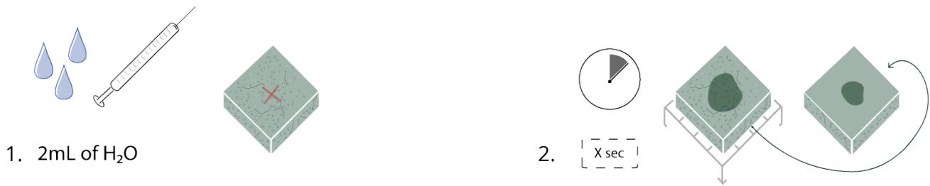
Figure 43. Diagram illustrating the testing process of the permeability test.
