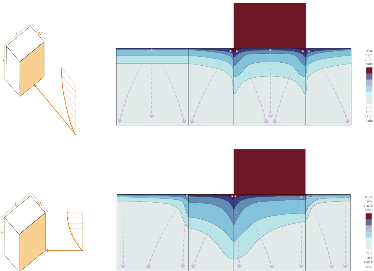
Figure 102. Wind-driven rain impingement pattern formed for the case of principle wind, for the simplification of a stand-alone building, firstly falling onto the façade's centre (upper diagram) and secondly on the building's corner (lower diagram). The arrows in the unfolded elevations, symbolize the main direction that the meso-scale curves should direct the water, with alternating flows to ensure a slow velocity for the best absorption conditions.
