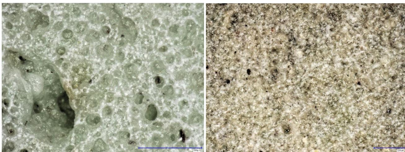
Figure 57. Microscopic images of TC06 & TC09, at different zoom scales (x100 & x50), depicting the effect of higher temperature in the chemical reactions of the additives during foaming. Various kinds of particles are still apparent with different colours.
