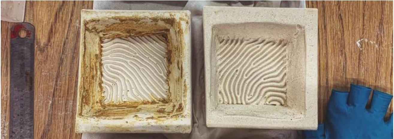
Figure 96. Image of two moulds, -one with clay traces of the inverted 3d-printed shape stabilized for pouring of the crystal cast mixture and the other cleaned- captured while bio-host glass mixtures were being demoulded after foaming. Image Source: Own.
