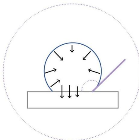
Appendix\_Figure 9. Diagram illustrating the measurement of the contact angle of the liquid to the surface, when there is a low attraction between the solid and the liquid and the surface tension of the droplet is stronger
