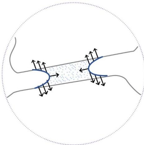
Appendix\_Figure 10. Diagram illustrating the typical meniscus shape of water inside a pore and its centre drawn inwards.
