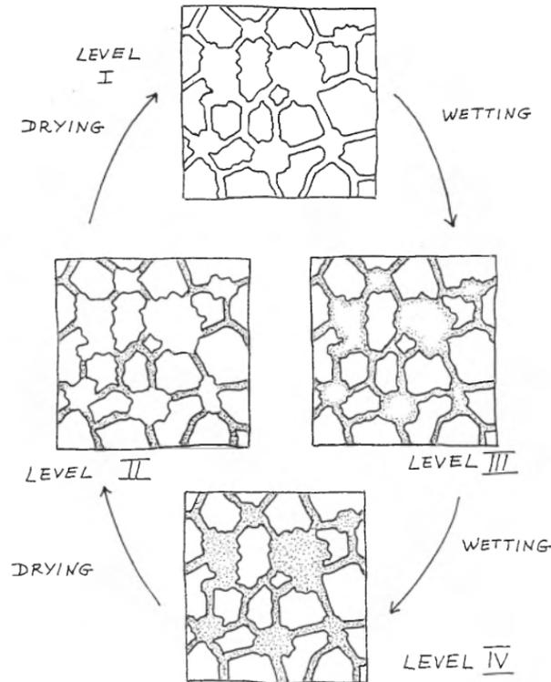
Appendix\_Figure 12. Diagram illustrating how the water moves inside a porous hydrophilic body. Image Source: page 10, Torraca, 1982.
