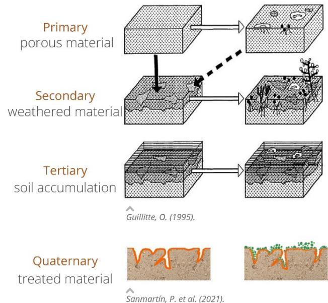
Figure 3. Bioreceptivity types depending on the state of the substrate material. These can all take place as a dynamic process attributed to the natural weathering, as the material deteriorates biofilm takes over with even more species. Image Source: Guillitte O. (1995) & Sanmartin P. et al. (2021).
