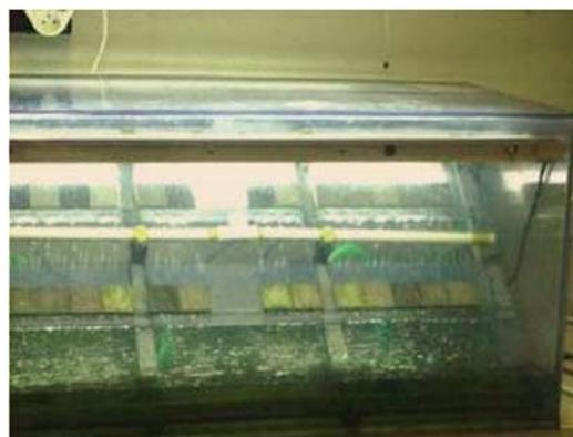
Figure 19. Experiment set-up for accelerated growth in inclination of 45° degrees. The first lamp provides lighting for the specimens, whereas the second for the nutrients and algae contained at the bottom with water being pumped constantly.
