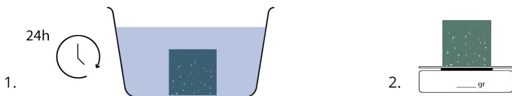
Figure 45. Diagram illustrating the water saturation level measurement.
