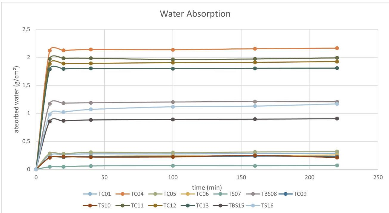
Chart 3. Water absorption curves for all the cubic-shaped specimens. Measurements taken after the shown time-period were excluded because they did not portray any specific difference.
