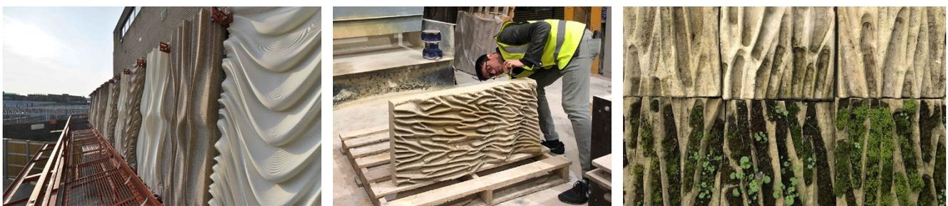
Figure 18. From left to right: a) The concrete pilot models of 1:1 scale, b) preparing the panel for St Anne's Catholic Primary School, c) samples exhibited in the Meanwhile Wildlife Gardens and Camley Street nature Park in London.
