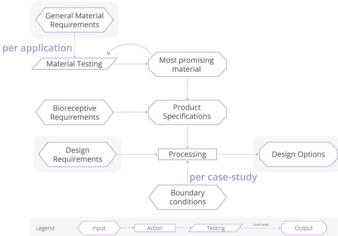
Figure 88. Engineering process for testing the upcycling bio-host glass and every new material to the design needs and bioreceptivity guidelines, to create a market application by adjusting the design according to the boundary conditions of each case study. Image Source: Own.
