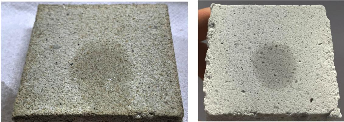
Figure 62. TBS08 (on the left) & TC13 (on the right) showcasing similar behavior of absorbing the water immediately, with different dispersion effects.
