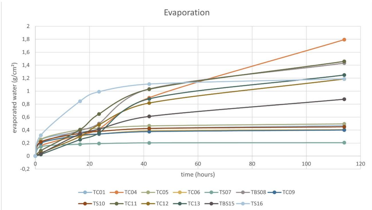
Chart 5. Evaporation rate curves formed from measurements taken during one-week period.
