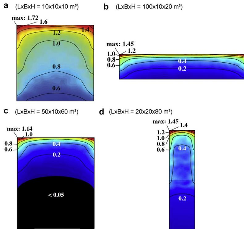
Appendix\_Figure 19. Catch ratio patterns along the analysed façade of the different building configurations, taking into account similar conditions as in Appendix\_Figure 16. Image Source: Blocken B. et al. (2013)
