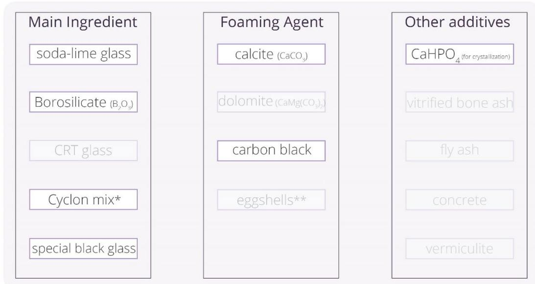
Figure 36. Different parameters related to the mixture's recipe, glass waste-foaming agent-additives. The list of values for each of them are an indication of what can be tested according to literature related both to glass foams and bioreceptivity.
