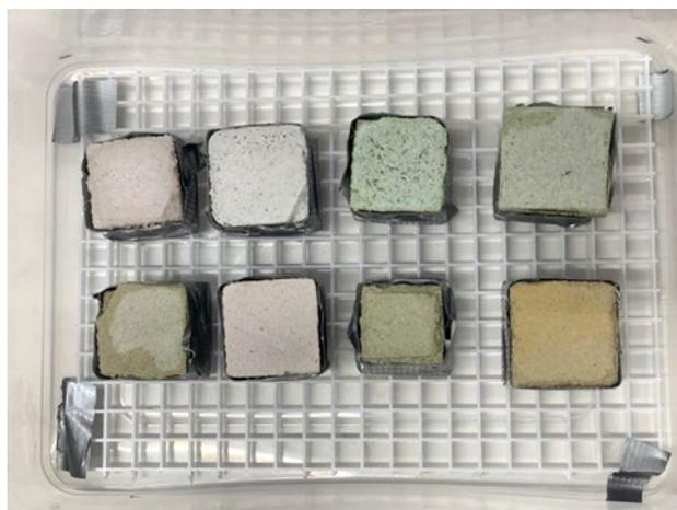
Figure 75. 1<sup>st</sup> batch of samples during the evaporation-rate testing. Uncovered surfaces have already started drying, from most of the specimens, except TC04 & TBS08. Image Source: Own.
