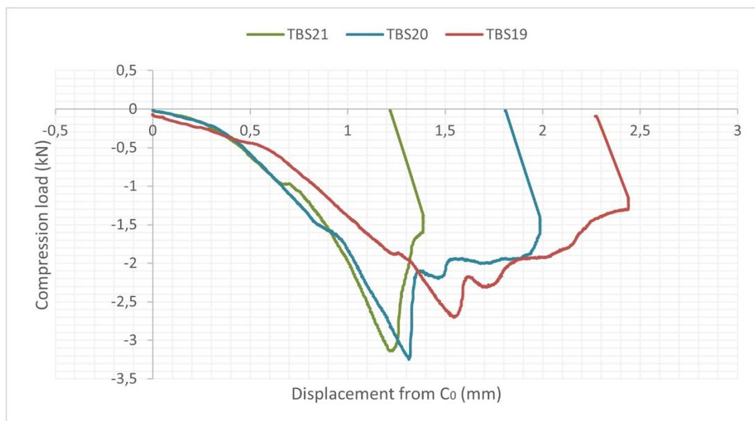
Chart 6. Load – displacement graphs for the three specimens of the same recipe [SLS powder (float glass) + Borosilicate cullet + carbon + CaHPO<sub>4</sub>, 790°C (2hrs), fast cool to anneal. point (1hr)]. Test conducted on 07/06/2022 together with Maiko van Leeuwen, using Istron 8872, in microlab, TU Delft.
