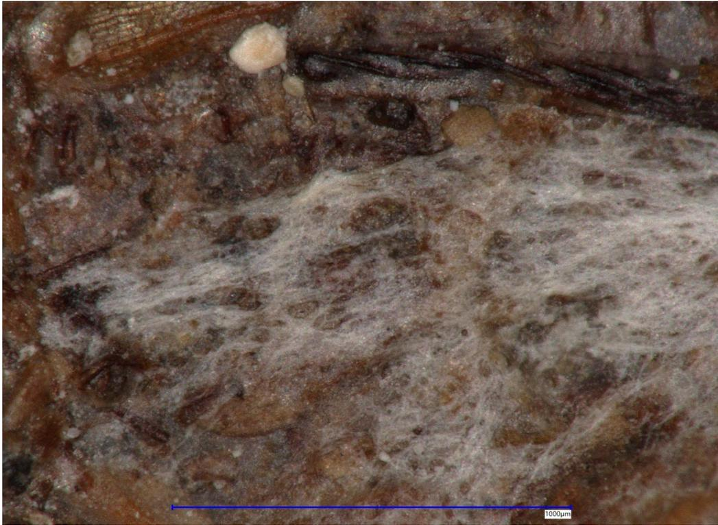
Appendix\_Figure 2. Fungi formation during moss-growth test conducted by Dimitrios Ntoupas on the mortar mixture presented in Appendix\_Figure 1. Potential reasons for this phenomenon, are the extreme lack of sunlight and samples-sealing from natural ventilation.
