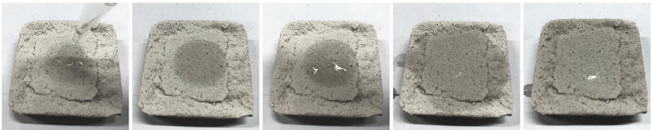
Figure 69. Timeframe from testing the sample TBS15, showcasing the low contact angle and therefore, high potential for water absorption along the whole thickness of it.
