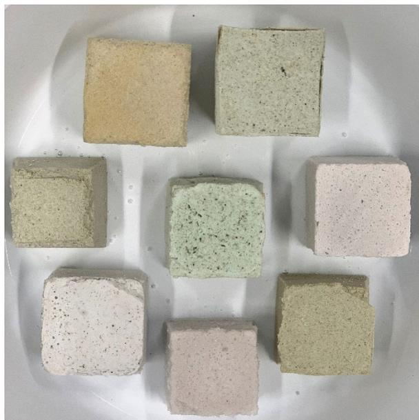
Figure 73. Specimens (TC01, TC04-TC06, TS07, TBS08, TC09, TS10) submerged into the water for 24hours to measure their weight after reaching their full-water saturation point.
