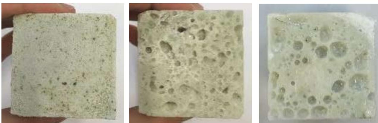
Figure 24. Photograph of samples with coded names: (from left to right) S-D01, SB-A01, SB-G01. Indicating the mixtures of soda-lime glass, soda-lime and borosilicate in different firing temperatures: 970, 1120, 1200°C. These samples indicated the highest porosity out of the tested recipes.
