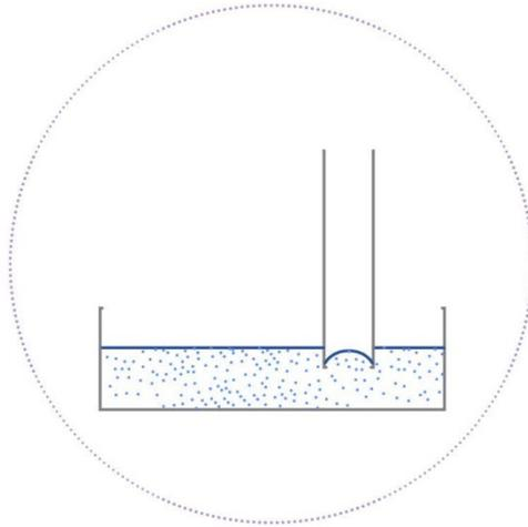
Appendix\_Figure 14. Diagram showing how water does not exhibit capillary rise on hydrophobic surfaces, an inverted meniscus is formed and there is no suction observed.
