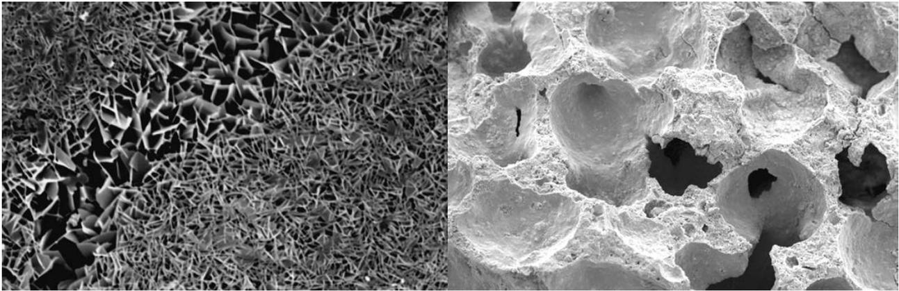
Appendix\_Figure 7. From left to right: a) High magnification view of microstructure of AAC material with bulk density 450kg DIA m-3 linear mesopore filled with crystalline tobermorite running between regions of microporosity. Scale bar 20 $\mu$ m. SEM image by Andrea Hamilton. b) Low magnification view of the coarse structure of a fracture surface of AAC showing aeration pores. Scale bar 0.5 mm. SEM image by Andrea Hamilton.
