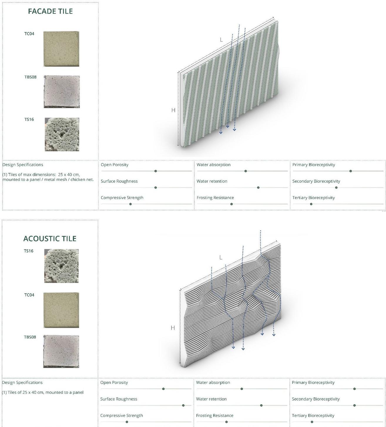
Figure 95. Boards for the recommendations of a façade and an acoustical tile, showcasing the different demands for material and bioreceptive properties, matching accordingly with the most relative specimens, created in this thesis.
