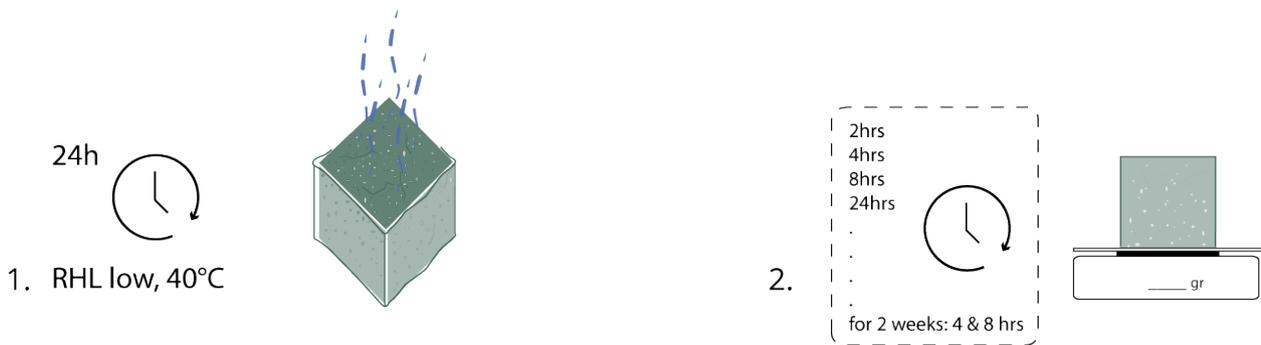
Figure 46. Diagram illustrating the evaporation test process, starting from the full-saturated point, aiming to reach the dried weight levels.
