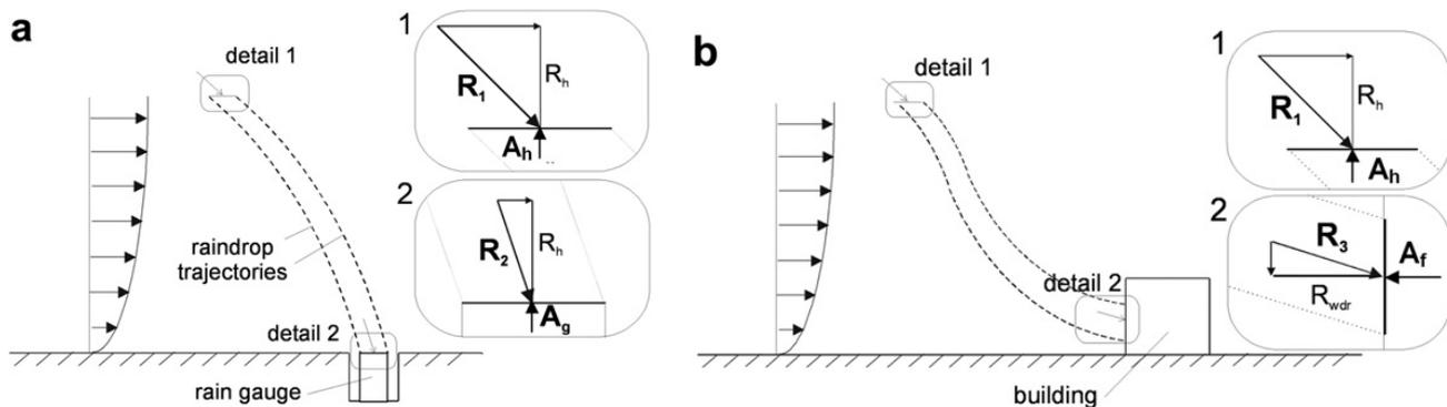
Appendix\_Figure 15. Wind direction and speed altering the rainfall in different conditions. (a) when there is homogeneous wind, the raindrop trajectories are parallel, (b) while when falling on a building they are not because in different heights the wind speed alters. Image Source: Blocken B. et al. (2013).
