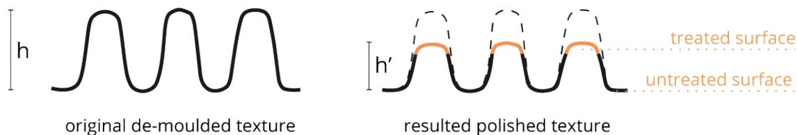
Figure 98. Diagram illustrating the original and obtained texture in section, after attempting to polish the tile shown in Figure 97. Image Source: Own.
