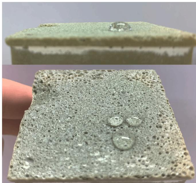
Figure 64. Highest contact angle observed, on a sample produced by T. Bristogianni, out of foaming Borosilicate glass.
