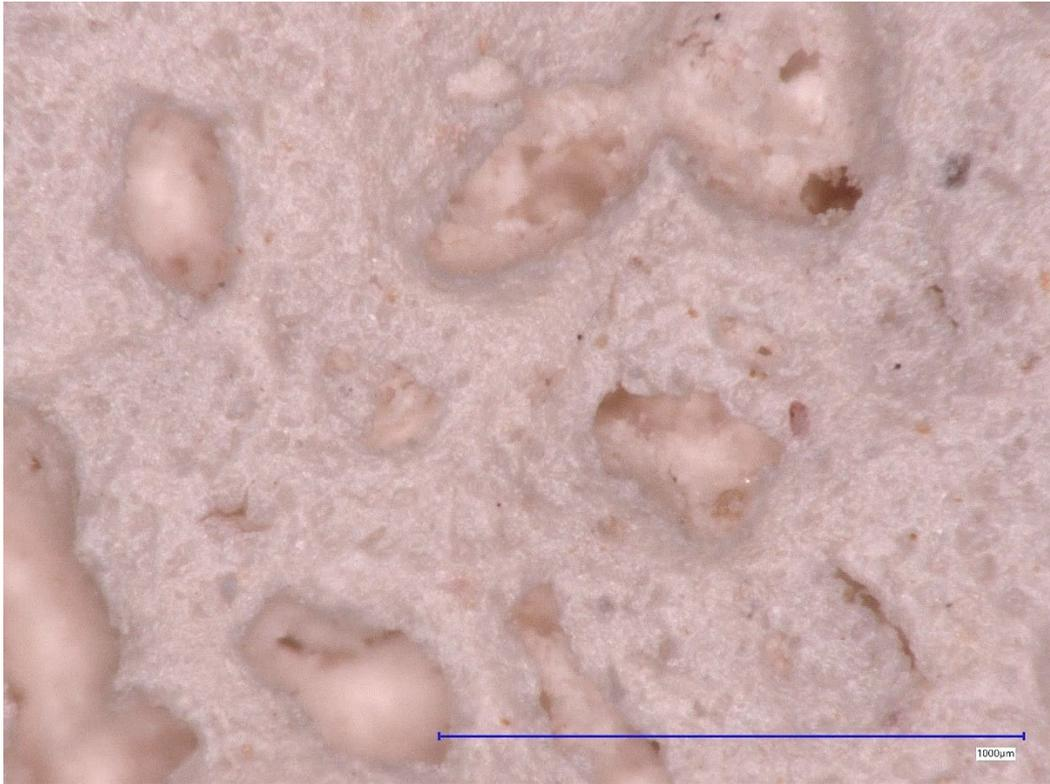
Appendix\_Figure 6. Microscopic image taken on 09/06/2022, commercial clay sample treated on the surface with coffee beans produced during Bucky lab course by Verhaagen B., V. , D. , Paszek W.. The chosen manual treatment has increased the surface roughness of the commercial product, by revealing the network of residual porosity underneath the outer layer, in which particles are bonded by water-mixing covering all the pores, but cracks.
