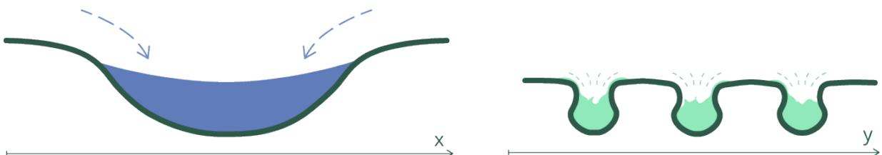
Figure 83. Diagrams expressing main design principles regarding bioreceptivity, emphasizing that these formations should take place in different directions. The left diagram showing the importance of directing water, therefore corresponds to a horizontal section, while the image on the right depicting a pocket-formation for the anchorage of microorganisms and capturing water in a vertical section. Image Source: Own.
