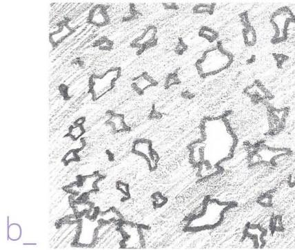
Figure 50. Distinctive microstructure type 01 of closed porosity. Sample TS07 & TS10 both consisted by Soda-lime glass, the first out of refined powder, foamed at 960 °C, while the second out of small cullet ranging between 200-400µm, foamed at 790 °C, showcase a complete different image of porosity and brittleness behaviour.
