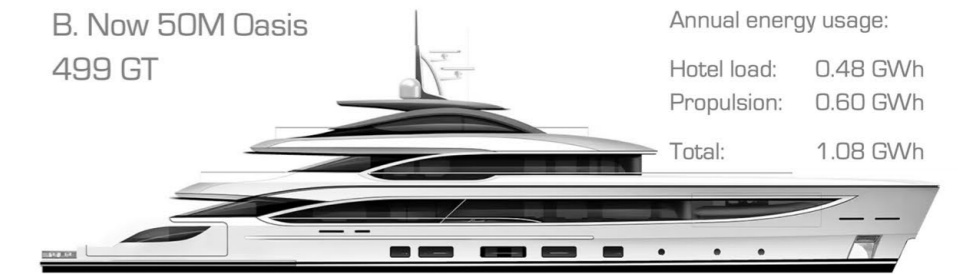
Figure 57: B. Now 50m Oasis by Benetti specs and energy usage (estimated with the method described in chapter 2.1).
