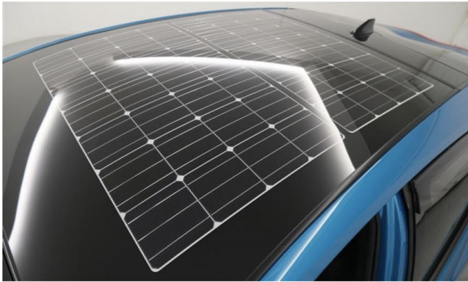
Figure 18: Example of curved glass solar panels used in a car roof (Solar Roof on Kia Sorento, 2025)
