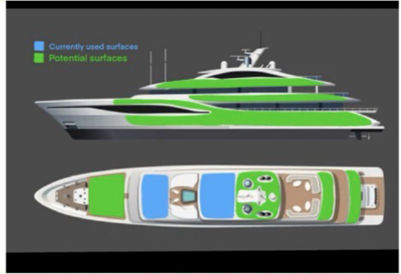
Image / figure 1 Illustrative example of used and potentials surfaces for solar cells. source: Adobe stock
