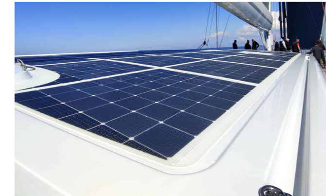
Figure 16: Example of a flexible stick-on panel mounted on a hard top of a Baltic 146, PATH. (Solbian Solar, 2022)
