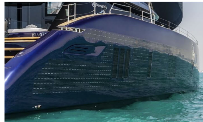
Figure 22: Example of solar cells integrated in the composite hull of a Sunreef 80 ECO. (SuperYachtTimes, 2022b)
