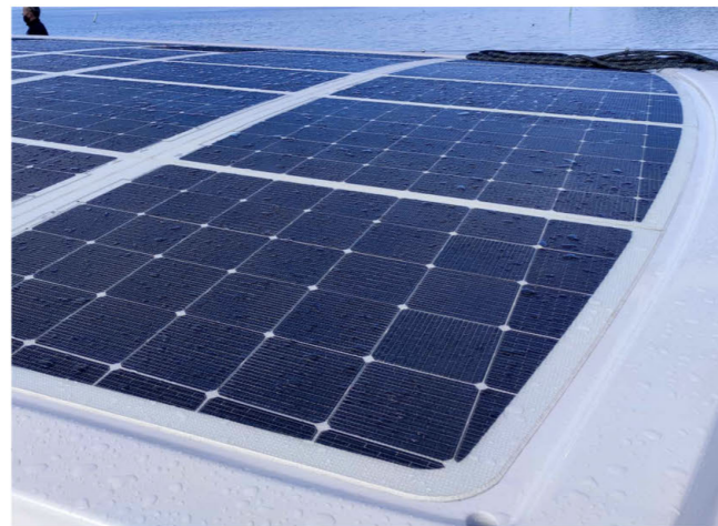
Figure 30: Solar panels that conform to the surface with the help of dummy cells (Solbian Solar, 2022)
