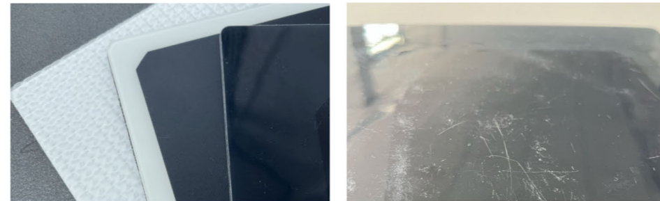
Figure 24: Left: samples with different textures, right: visible wear on the top surface. Samples provided by Solbian
