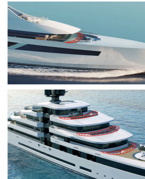
Figure 42: Comparison between low-profile and multi-deck yacht designs in terms of loss effective horizontal PV surface area
