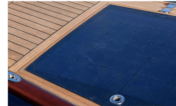
Figure 15: Example of a flexible stick-on panel mounted on a teak deck of a Spirit 44CR. (Solbian Solar, 2021)
