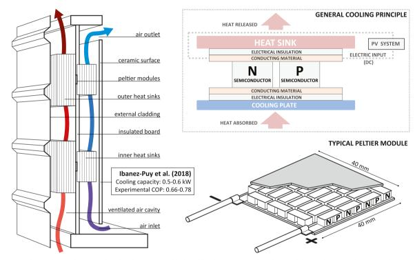
Fig. 2. Thermoelectric cooling façade prototype developed by Ibanez-Puy et al. and general thermoelectric cooling principle.
