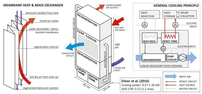
Fig. 6. Integrated small-scale membrane based LDAC unit developed by Elmer et al. and liquid desiccant general cooling principle.
