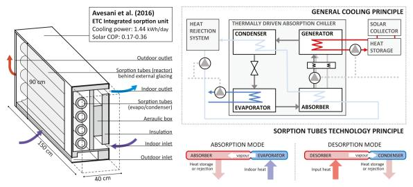
Fig. 3. Integrated sorption collector & sorption tube technology developed by Avesani, Hallstrom et al., and general absorption cooling principle.
