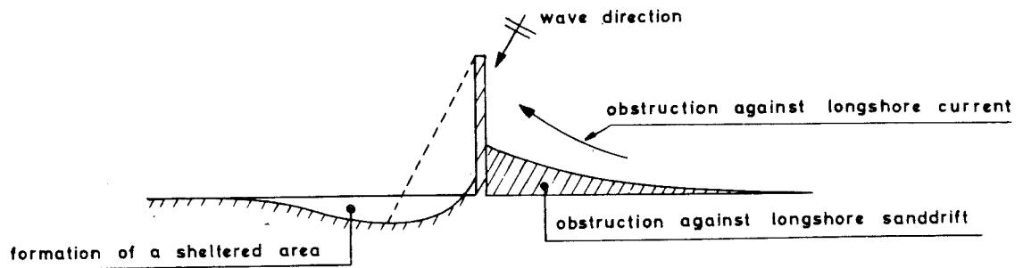
Fig. 8 The effects of the construction of a groyne
