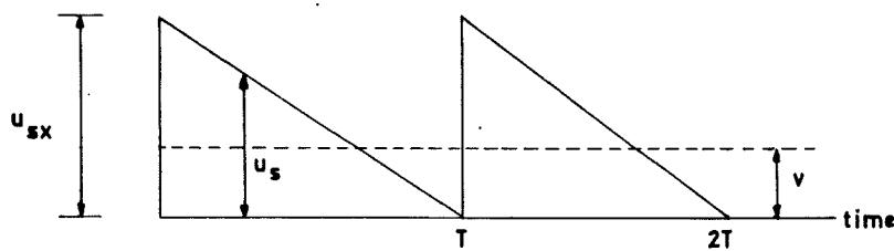
Fig. B 1<sup>a</sup> Variations in longshore water velocity  $u \sin \varphi$  according to EAGLESON
