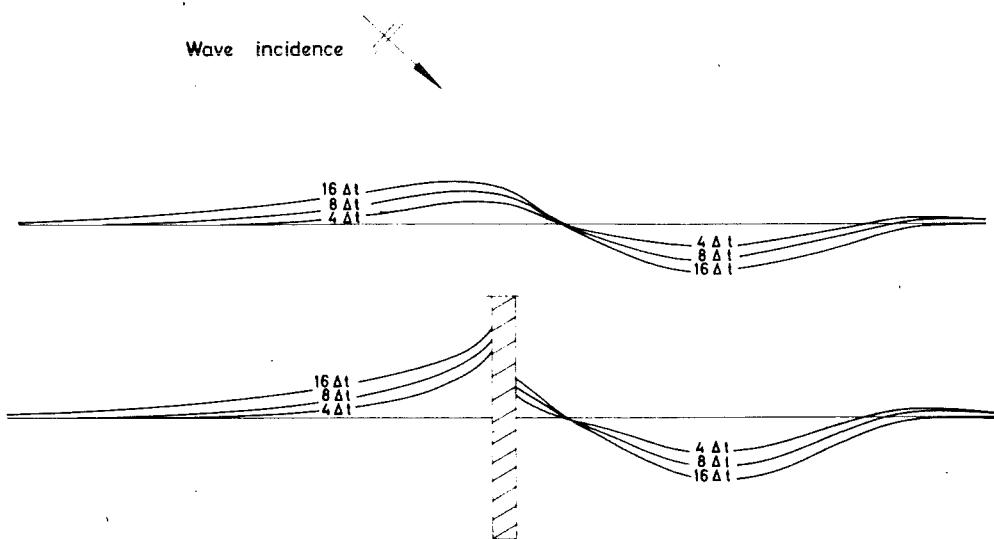
Fig. 15 Accretion and erosion near a groyne, numerical solution with diffraction (two-line theory)
