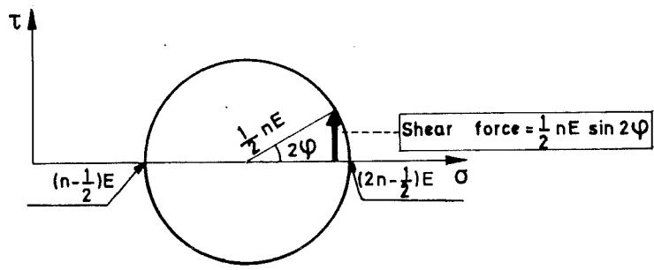
Fig. 4 Mohr circle, representing the radiation stress.
