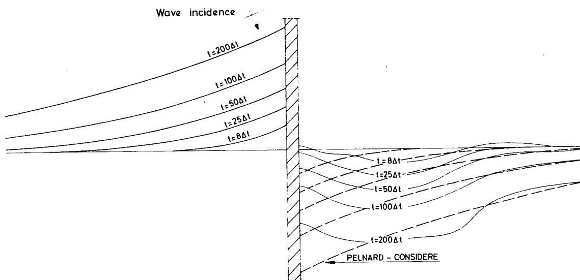
Fig. 11 Accretion and erosion near a groyne, numerical solution with diffraction (one line theory). The dotted lines at the right hand gives erosion according to Pelnard - Considerere.
