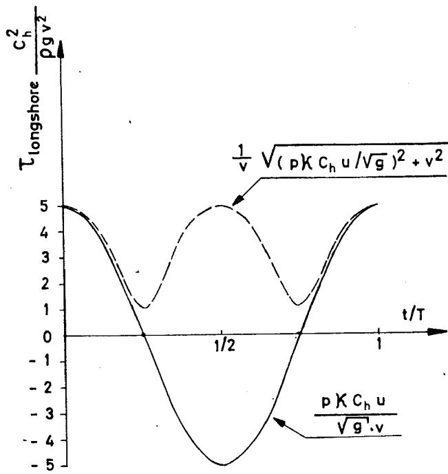
Fig. 2  $\bar{\tau}_{\text{longshore}}$  and orbital velocity as function of  $t/T$
