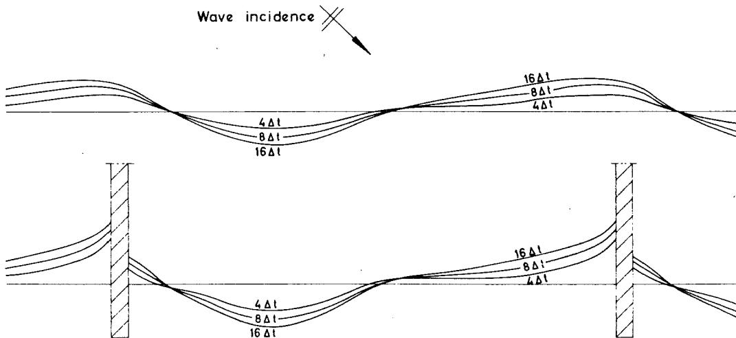
Fig. 16 Behaviour of beach and inshore between two groynes.(two-line theory)
