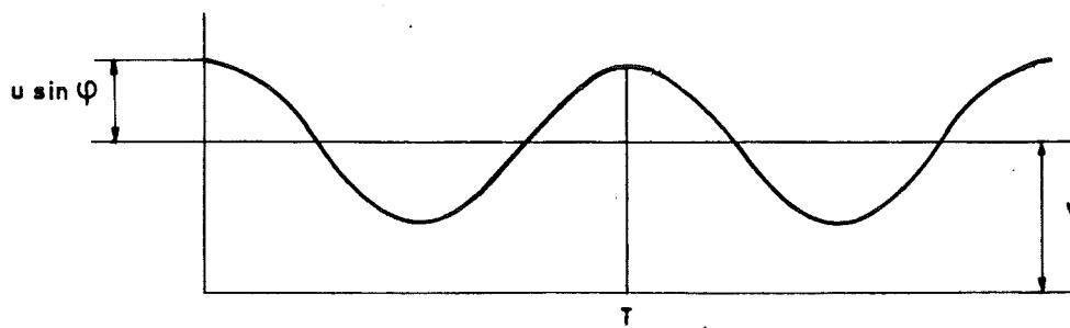
Fig. B 1<sup>b</sup> Variations in longshore water velocity  $u \sin \varphi$  according to BAKKER
