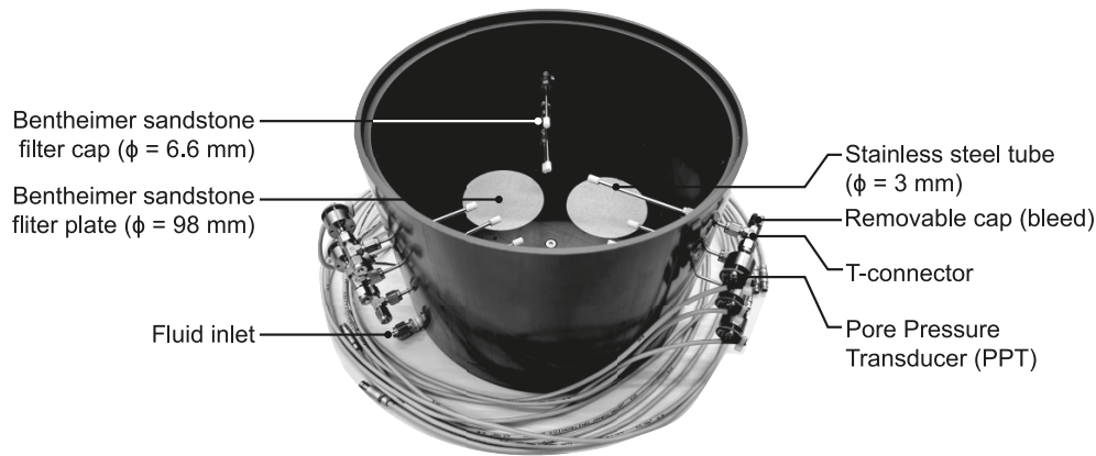
Fig. 4. Instrumented strongbox, equipped with nine pore pressure transducers (PPTs) positioned at fixed depths and radial distances relative to the model centroid. The base of the strongbox contains a removable 15 mm thick insert fitted with four Bentheimer sandstone filter plates to facilitate uniform sample saturation while flushing fluid through the inlet at the base of the strongbox.
