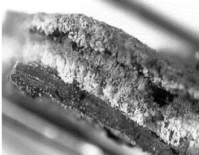
Figure 2-3: Different ash layers on a superheater pipe (from the CHP plant Uppsala/Vattenfall).
