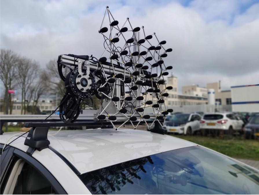
Figure 4.1: The microphone array used in the collection of dataset used in this thesis. Multiple microphones was used in the collection of this dataset as it was used in the implementation of localization based approach.
