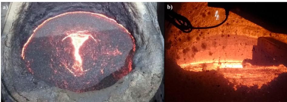
*Figure 1.2: a) Slag in a hot metal ladle prior to HMD. b) Slag skimming at an HMD station (photos: Alison Tuling, 2020).*
