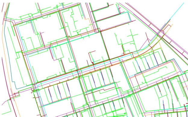
Figure 3. Representation of the input datasets used in this work. Electrical network (in red) and sewer-system network (in purple) of the city of Rotterdam.
