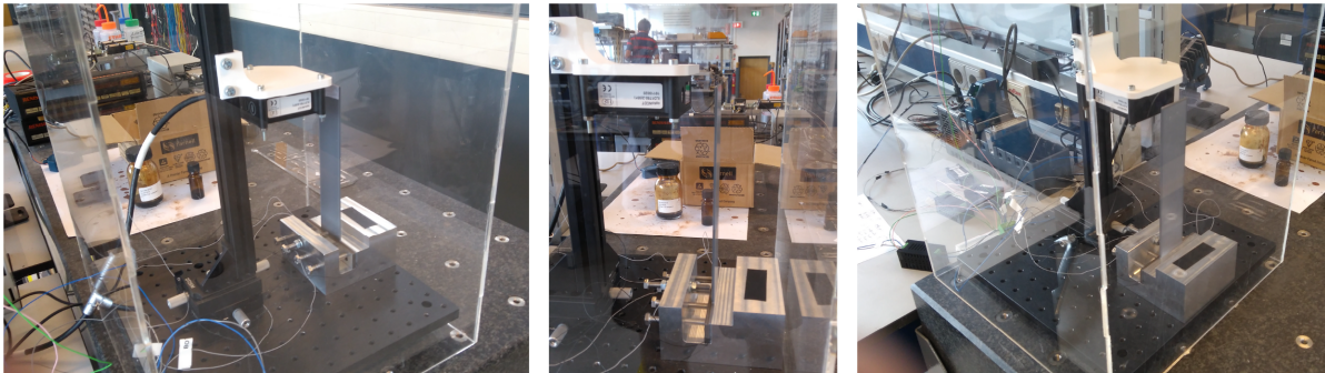
Figure 5.8: Shows the flexure in the experimental setup. Do note the white paper on top of the flexure facing the laser distance sensor (OptoNCDT 1750), the paper is used to aid the laser sensor.
