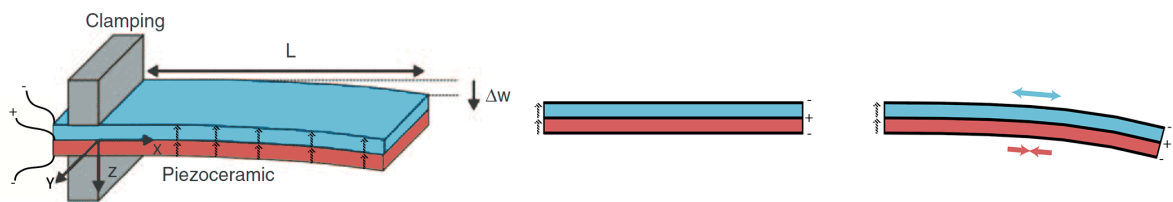
Figure 3.22: Left) Bimorph Bender Actuator [26]. Angle-dashed arrows show polarization. Right) shows how the bender works. Blue is extending, and red is contracting piezo.
