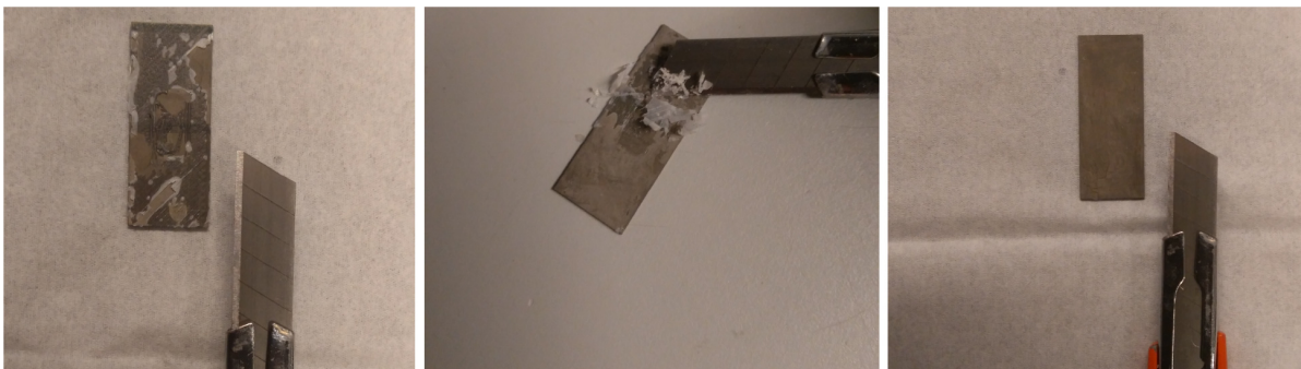
Figure C.23: Shows how the epoxy is scraped off a piezo actuator. In the end the actuator is cleaned and scrubbed with isopropanol.
