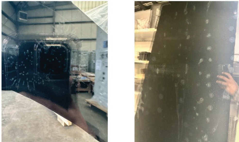
Fig 28. Air bubbles from the application of a safety film
