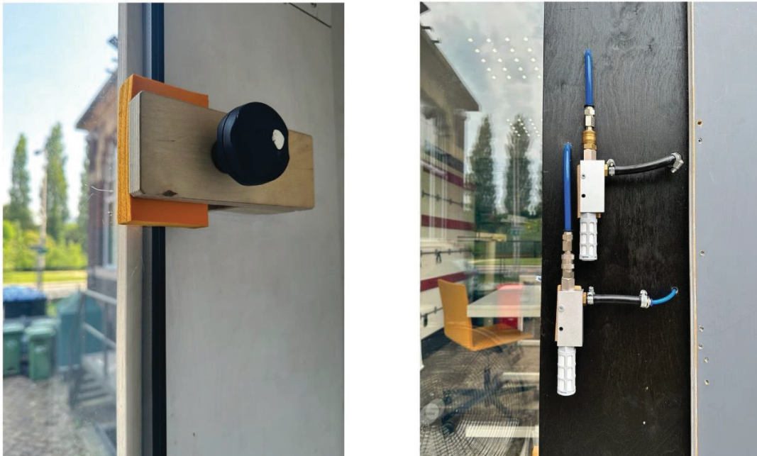
Figure 47: Fixing mechanism on the van and vacuum generator
