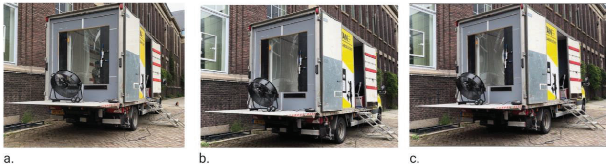
Figure 53 Outdoor view during the deflection of the glazing: a. condition with no deflection, b. condition with deflection 10 mm; c. condition with maximum deflection at 23 mm.
