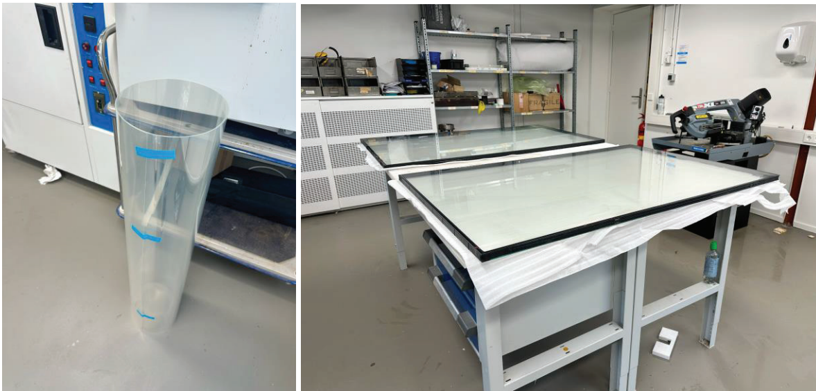
Figure 27: Safety film (left) and safety film application finished and when the glass is left to dry (right)
