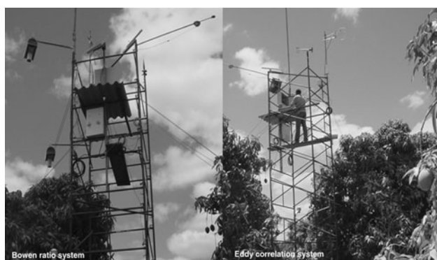
Fig. 1 Energy balance measurement systems in mango orchard, Petrolina-PE, Brazil
