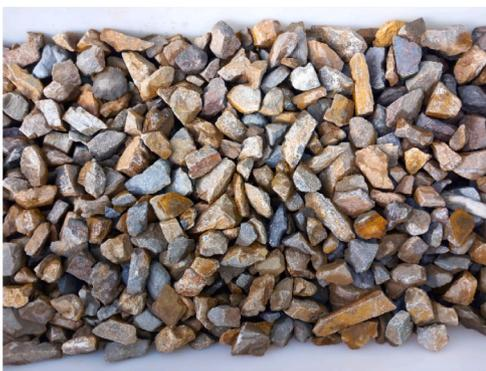
**c** Clean ballast particles in the reservoir: AREMA
