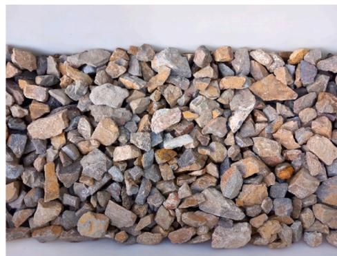
**d** Clean ballast particles in the reservoir: AREMA
