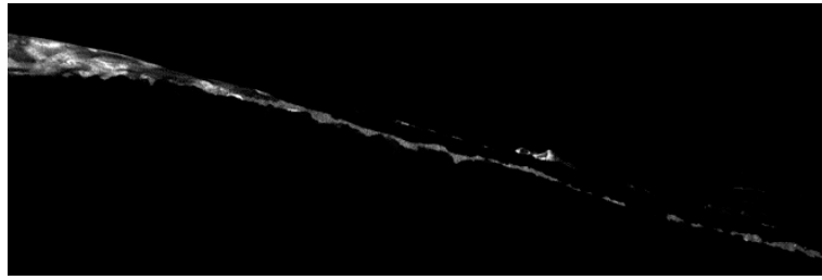
Figure H.2: Raw frame of the field of view during PIV measurement of h = 3.6 cm. Flow over the structure at the lower part shows a dark area with no particles.
