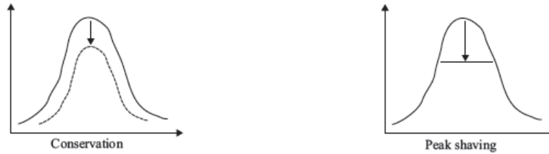
Figure 20: Energy conservation and peak shaving shaping objective, source: Lund et al. (2015) and Gellings & Smith (1989)
