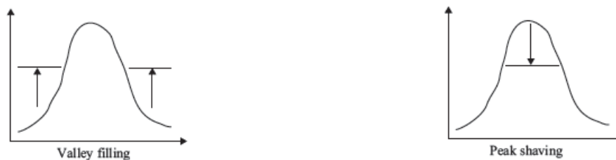
Figure 24: Valley filling and peak shaving shaping objectives, source: Lund et al. (2015) and Gellings & Smith (1989)
