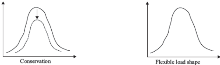
Figure 22: Energy conservation and flexible load shaping objectives, source: Lund et al. (2015) and Gellings & Smith (1989)
