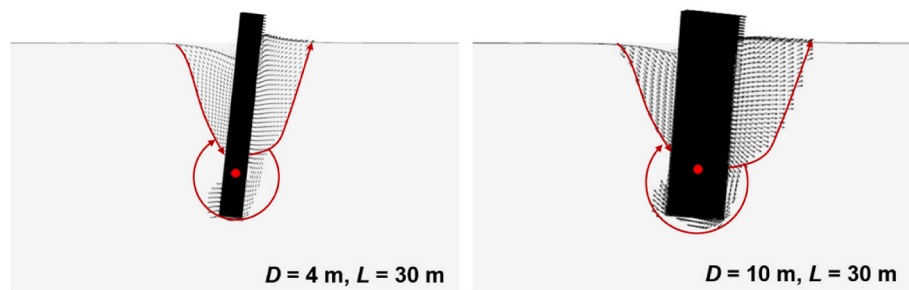
Fig. 10. Failure mechanism of the rigid monopiles in sand (Wang et al., 2022b).
