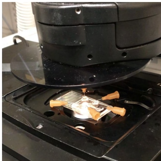
Figure 5.12: The LOC device placed in the sample holder of the Leica SP5 confocal microscope
