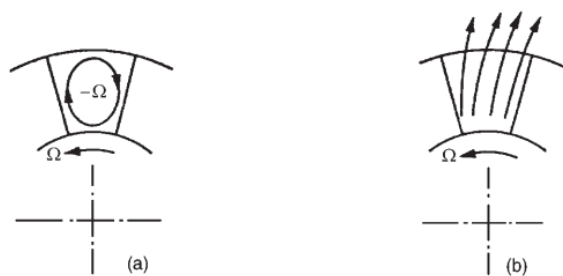
Figure 2.8: (a) Relative eddy without any through flow. (b) Relative flow at impeller exit (through flow added to relative eddy) , obtained from Dixon (1998)
