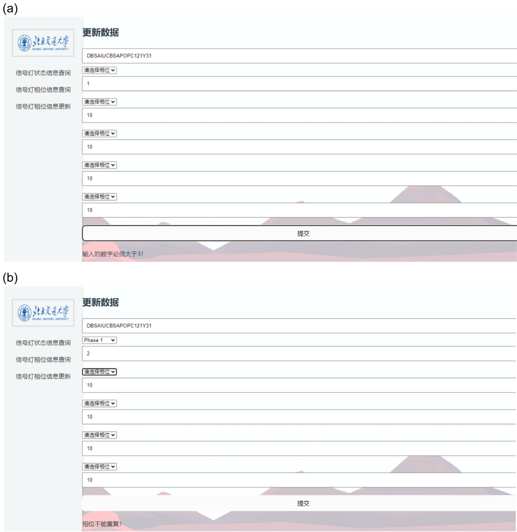
FIGURE B7 (a) Frontend phase information update interface. *Warning message of phase period length (b) Frontend phase information update interface. *Warning message of phase number input.
