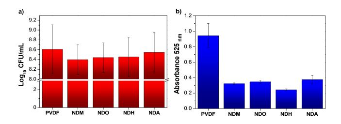
**Figure 8.** Antimicrobial activity of the pristine PVDF and ND/PVDF films (2 wt.%) measured using: a) CFUs (colony forming units) of *E. coli* growing in suspension over the nanocomposites and b) the total biomass growing on material's surface assessed by crystal violet assay.
