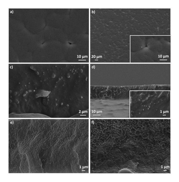
Figure 2. SEM micrographs of the surface of a) NDH 0.5 wt.%, b) NDM 2 wt.% and the cross section of c) NDO 0.5 wt.%, d) NDA 2 wt.%, e) NDH 0.25 wt.% and f) NDM 2 wt.%.
