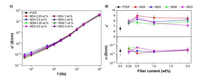
**Figure 6.** Electrical properties measured at room temperature: dielectric constant (a); dielectric loss (b); a.c. electrical conductivity as a function of frequency (c); dielectric constant (at 1 kHz) and d.c. conductivity as a function of filler content and type (d).
