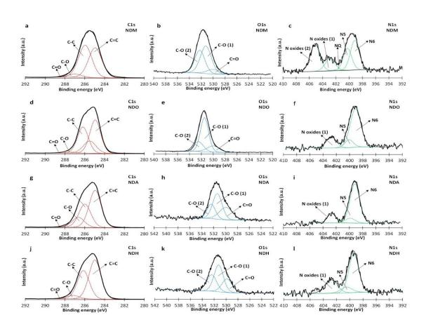
Figure 1. XPS spectra and deconvolution of C1s (a, d, g and j), O1s (b, e, h, k) and N1s (c, f, i and I) regions of the different ND samples: NDM (a-c), NDO (d-f), NDA (g-i), NDH (j-I).
