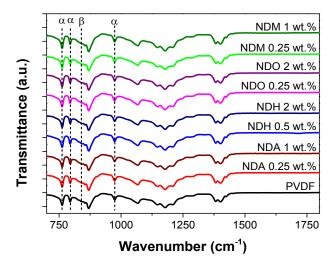
Figure 5. FTIR-ATR spectra of PVDF polymer and various ND/PVDF composites.
