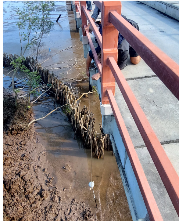
Figure A.15: Lowering the RTK from the pier
