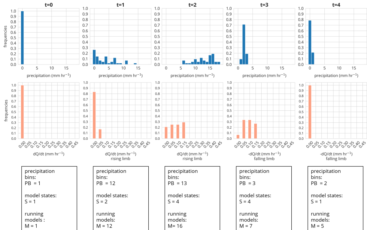
Figure 5. Binned precipitation field (blue) and binned model states (orange) of the adaptive model ( t = 0 ; 3 August 2014 15:00 CET). PB is the no. of allocated precipitation bins, S the no. of allocated model space bins, and M the no. of running models at the given time step. The spatial distribution of the precipitation and the model states for event I are displayed in Fig. 6.
