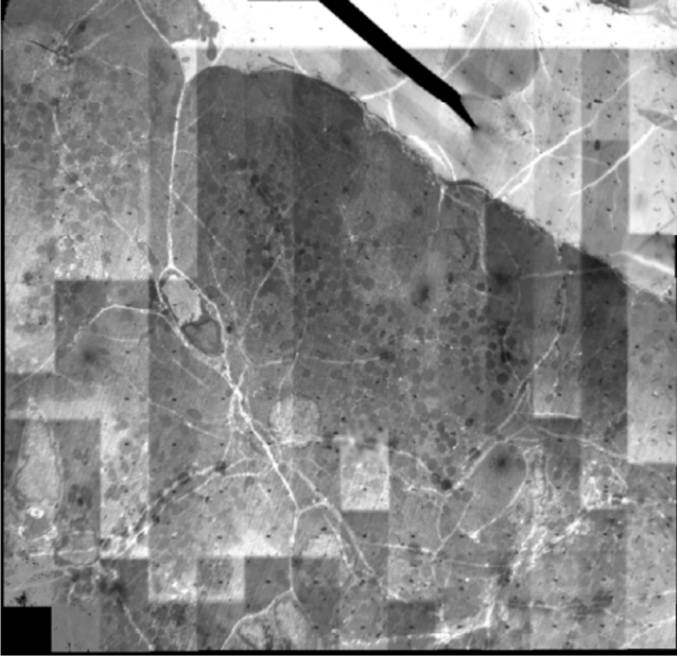
Figure 1.1: Image from Ren [2], showing transmission electron imaging of rat pancreas tissue in the TU Delft multi-beam prototype. The image shows a 14x14 beam image grid, imaged at a 15keV landing energy.
