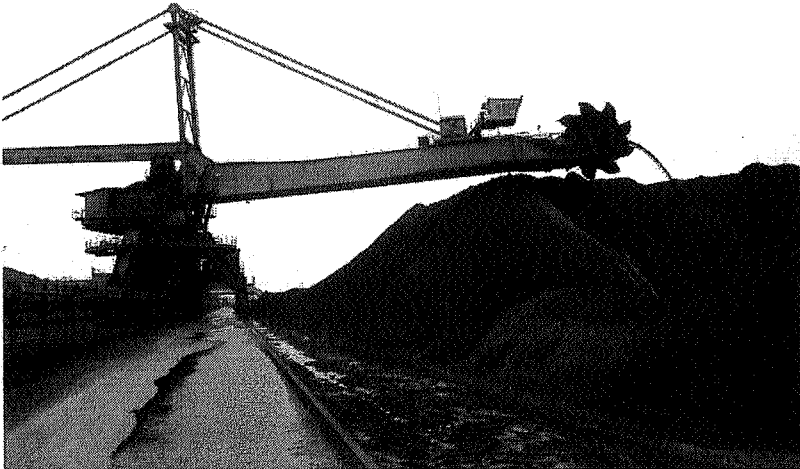
figure 4-7: Stacker-reclaimer (EMO-terminal in Rotterdam).
