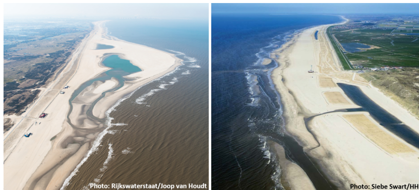
Figure 5.1: Aerial photographs of two large-scale nourishments in the Netherlands: the Sand Engine (left) and the Hondsbossche Dunes (right)
