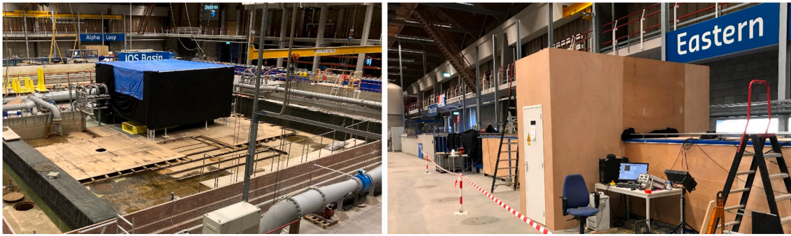
Fig. 1. Two examples of safety precautions that were taken at laser-based PIV measurements in the facility hall of Deltares to prevent risk of eye- and/or skin damage from laser light exposure. Left: a large tent of laser-safe shielding material in one of the scale model basins; Right: a wave flume with its PIV measurement section, which is completely shielded with multiplex plating.
