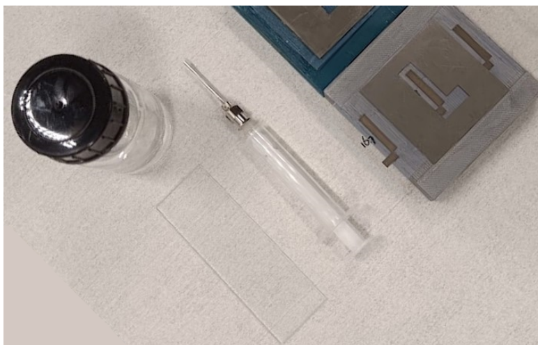
Figure 3. The stencil printing set-up. After completing the bottom electrode, the sample is placed between a magnetic block and a stencil (right). The polymer ink (glass bottle on the left) is loaded into a syringe (center), applied on the stencil, and wiped with a microscopy slide (bottom left).
