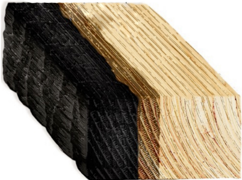
Image 11. Due to its combustion properties, timber creates a charring layer that protects the components during a fire.
