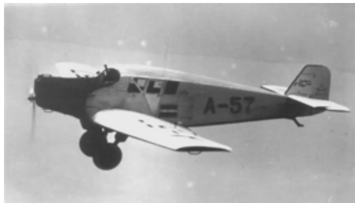
Figure 1.1: Photo of a Junkers F13, the world's first all-metal passenger aircraft, manufactured in Germany after World War I ( Courtesy of 1000aircraftphotos.com ).
