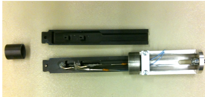
(c) Inside the afterbody: two pressure tubes glued to pressure ports.
