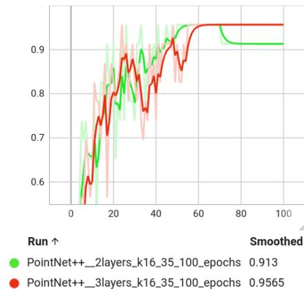
Figure 4: PointNet++ accuracy with three convolution layers (red) instead of two (green)
