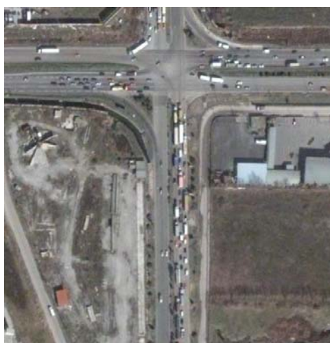
Figure 132 Traffic jam due to traffic lights where the bridge meets the NR [Google Earth]
