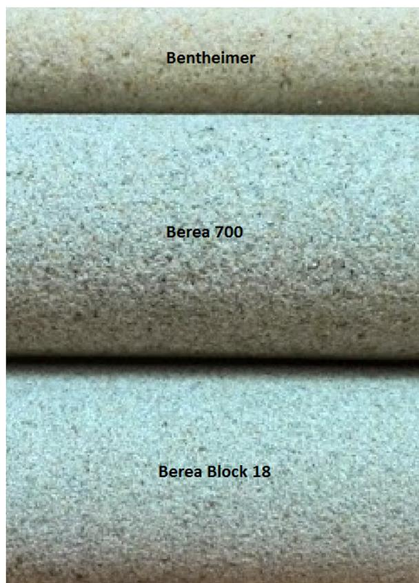
Figure 3.1: Three different core materials: Bentheimer, Berea 700 and Berea 18
