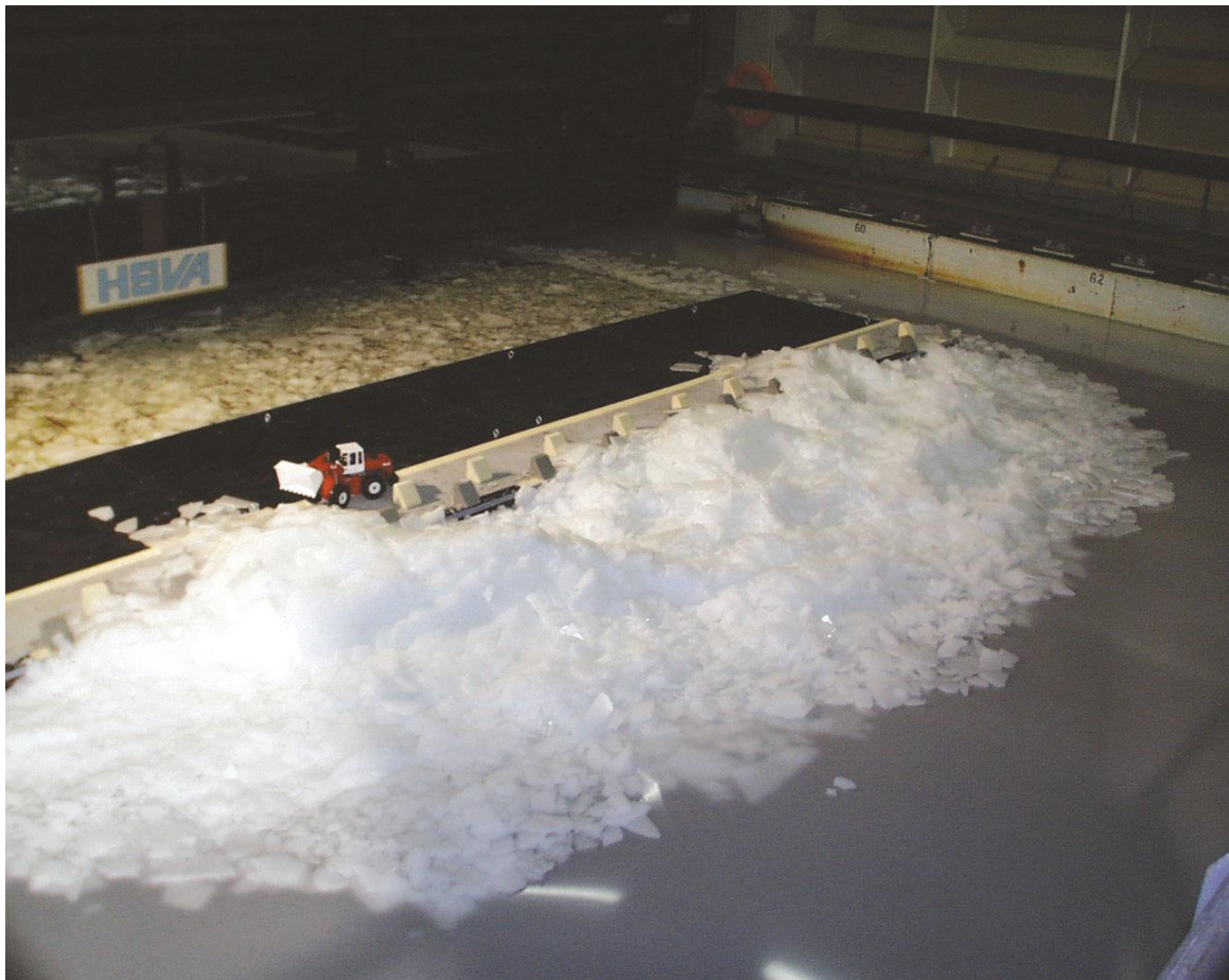
Fig. 9 Laboratory setup of ice-loading.
