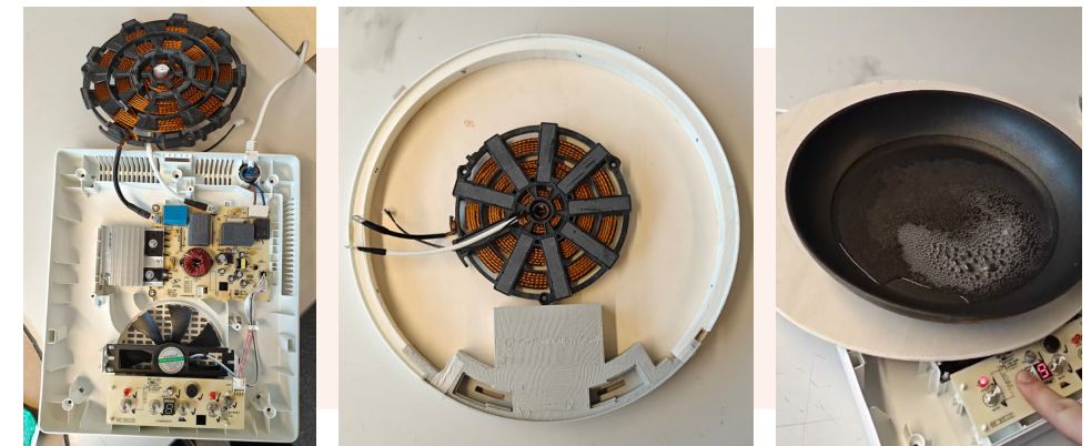
Existing induction plate Induction coil integrated in prototype Activating induction coil through wooden plate
