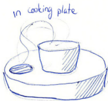
Figure 5.23 Top extraction of fumes
