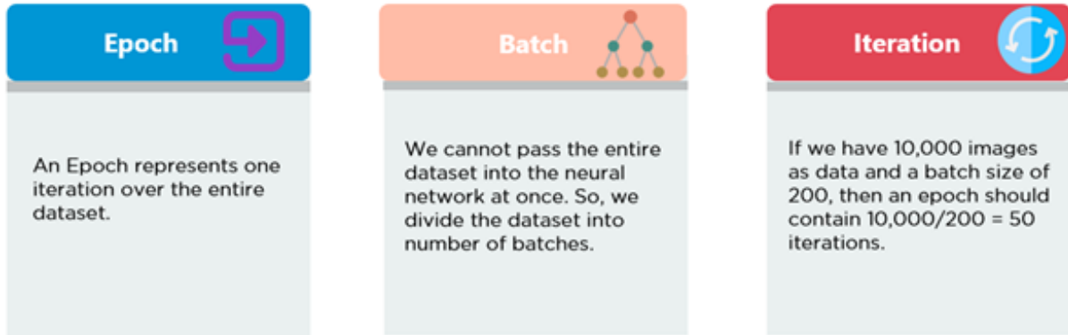
Figure (2.3) The number of training examples in the dataset and the batch size together decide the number of iterations required to complete one epoch. The figure is reproduced from an online blog post.
