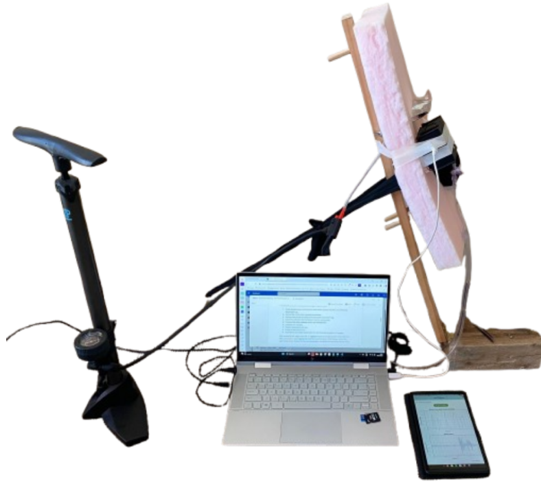
Figure 4.11: Experimental phantom validation setup with breadboard prototype positioned within the enclosure housing and connected to the pressure model while streaming data via BLE.
