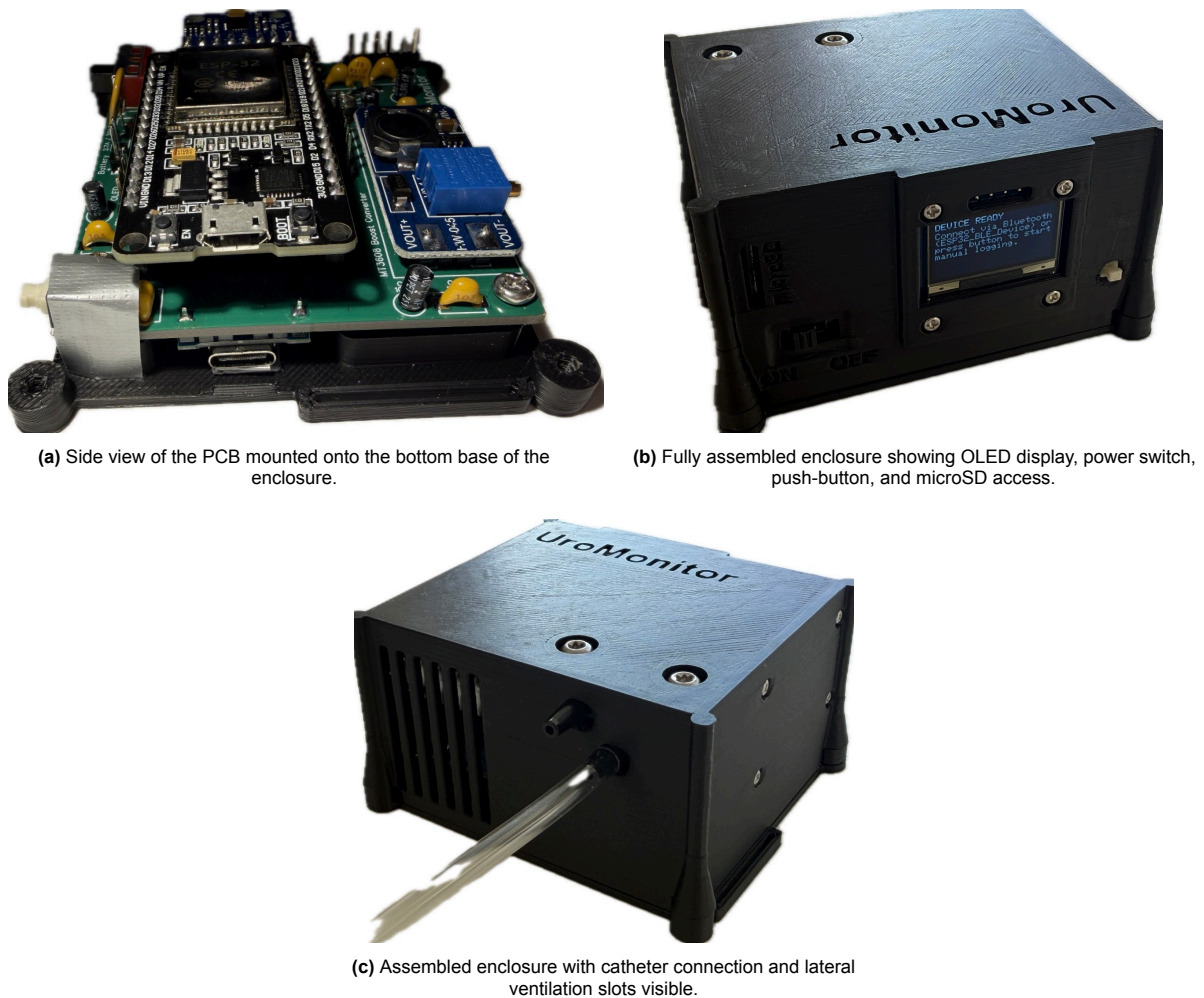
Figure 4.9: 3D-printed UroMonitor enclosure and internal assembly configuration.
