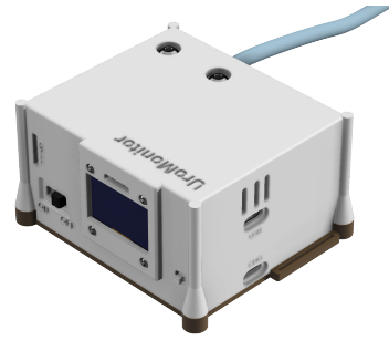
(b) User-interface view of the enclosure showing the OLED display, microSD card slot, latching push-button, and power switch. All user-facing components are oriented upward to maximise visibility and ease of access when the device is worn on the torso.
