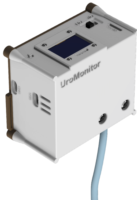
(e) Angled orientation view emphasising ergonomic alignment during wear. User-interfacing components (OLED display, microSD slot, and controls) are directed upward toward the user's head for visibility and interaction, while the catheter is routed downward, reducing bending stress and potential signal damping while improving concealment under clothing.
