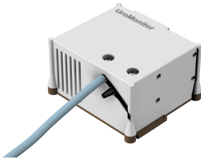
(c) Perspective view highlighting the catheter exit port, side ventilation slots, and microSD card module mounting holes.
